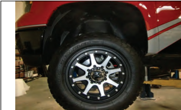
Install wheels/tires lower vehicle to ground check clearances
