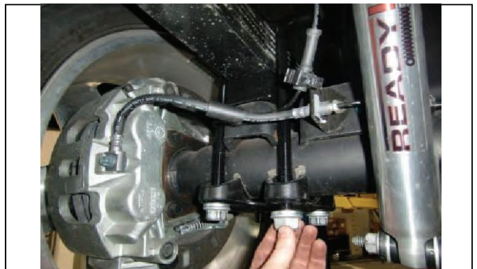
Install new longer u-bolts and install new hardware,
