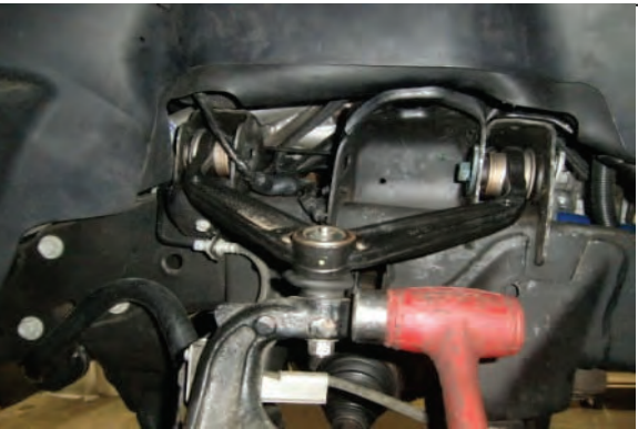
Strike spindle to disconnect ball joint from upper control arm
