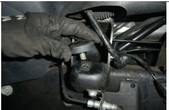
At forward control arm pocket attach clip and droop limiter.
