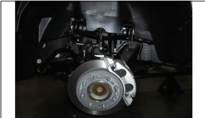
Securely lift vehicle and remove wheels
