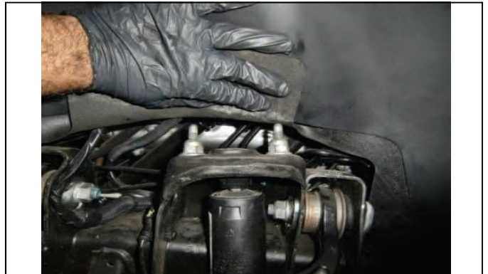
Push back soft fender liner to remove upper shock nuts.
