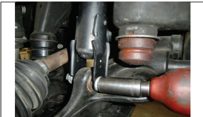
Loosen and remove lower shock hardware. New shocks req'd
