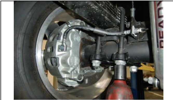
Loosen and remove u-bolt hardware
