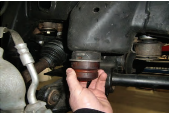
Remove factory lower control arm bump stops (4)
