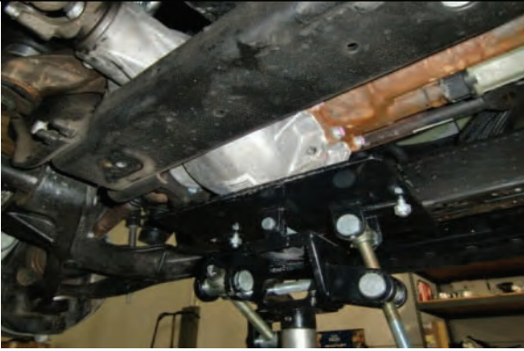
Support differential and remove differential mounting bolts
