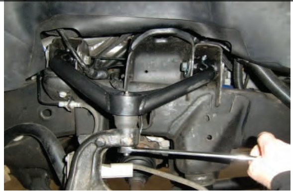
Connect upper ball joint to spindle
