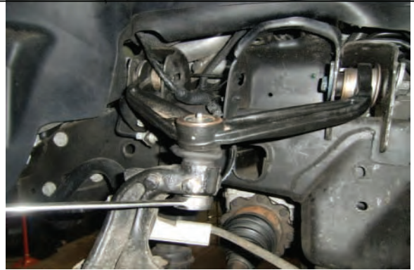
Loosen and remove upper ball joint nut.
