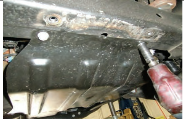
Reinstall front skid plate
