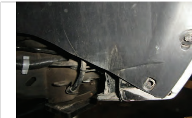
Slight/moderate trimming may be necessary for tire clearance
