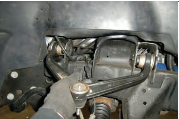
Remove upper control arm from frame pockets
