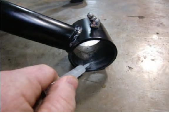
Install zerk fittings and apply grease to pivot tubes
