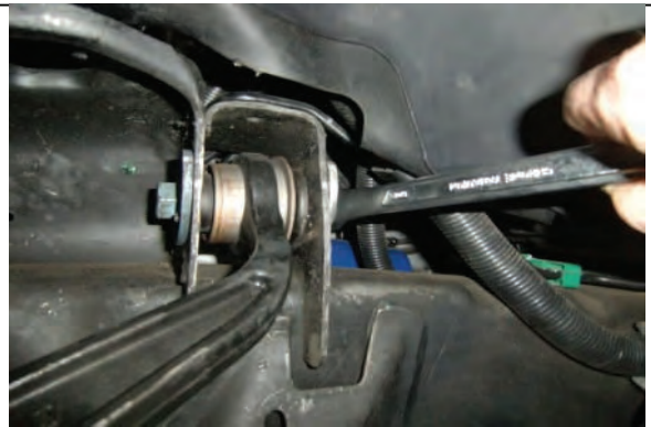
Loosen and remove pivot bolts and cams; they are very tight.
