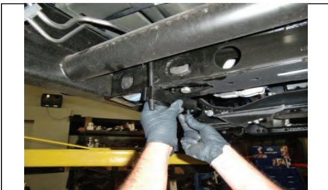
Position torsion bar unloading tool over cross member
