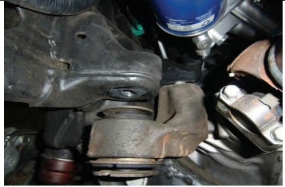
Remove (4) diff mounting bolts at frame, lower differential.
