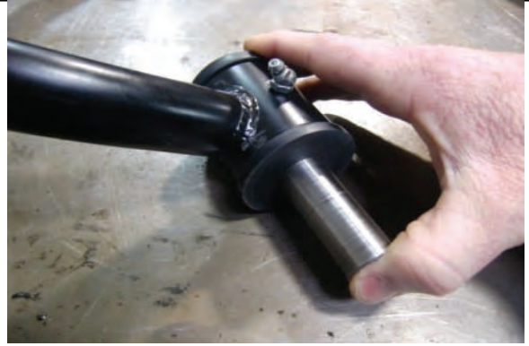
Assemble bushing halves and insert crush sleeves
