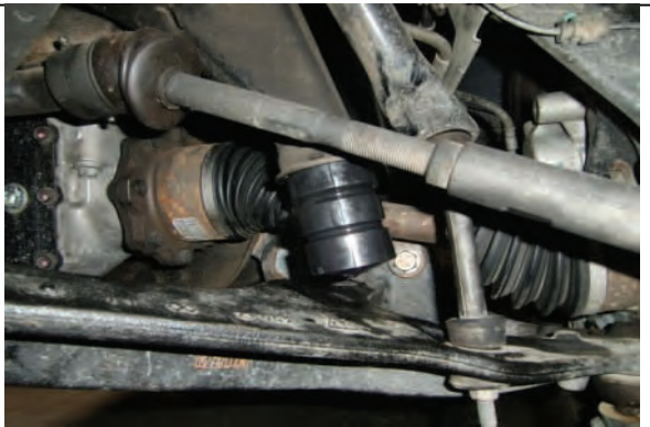
Install new provided bump stops (4) in OE locations
