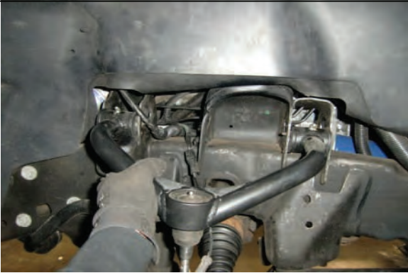
Install new upper control arm assembly with OE hardware
