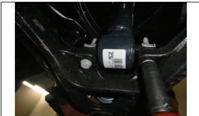
Remove lower strut mounting bolts
