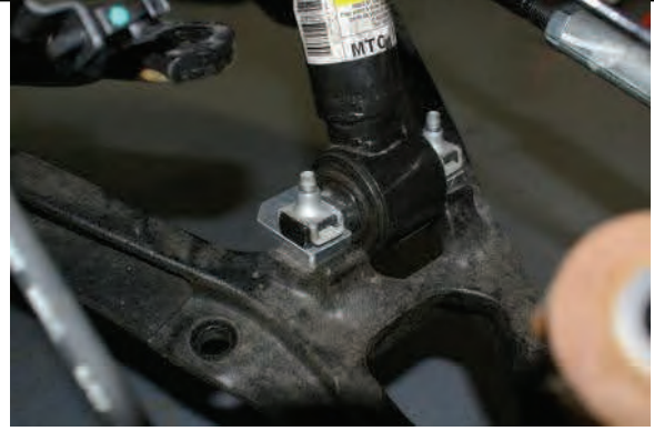
Install lower strut spacer and tighten,
