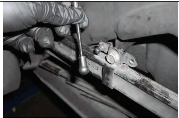
AUTORIDE ONLY: Carefully pry arm off trailing arm bracket
