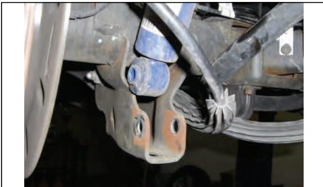
Disconnect Lower shock mounts
