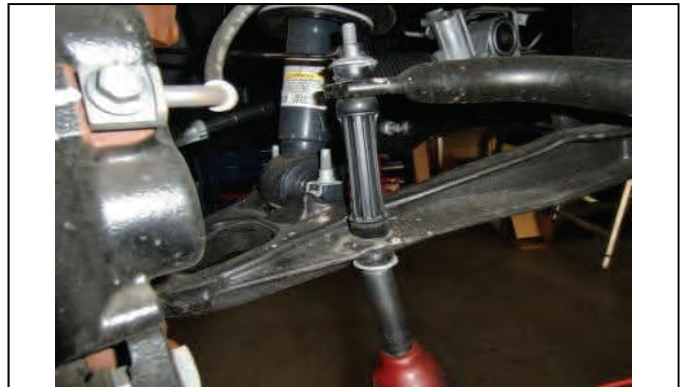
Disconnect dr/pass sway bar end links
