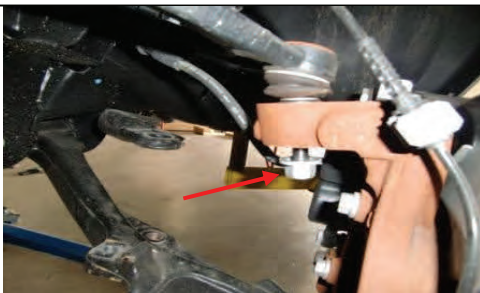
Support suspension loosen upper ball joint nut
