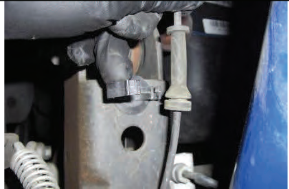
Unclip ABS lines at upper trailing arm
