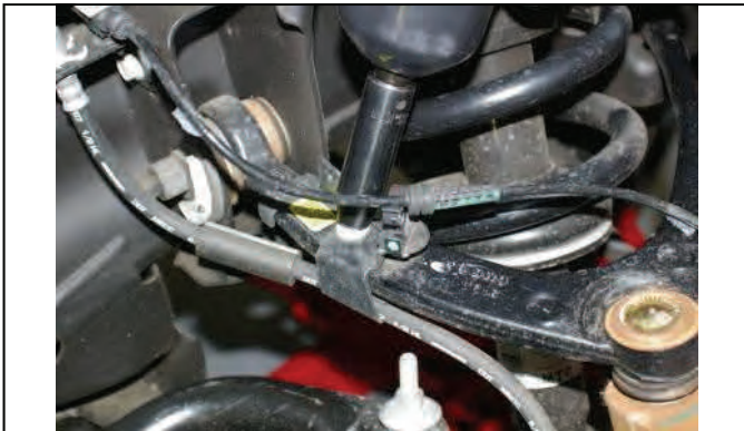
Disconnect ABS/brake bracket from upper control arm.
