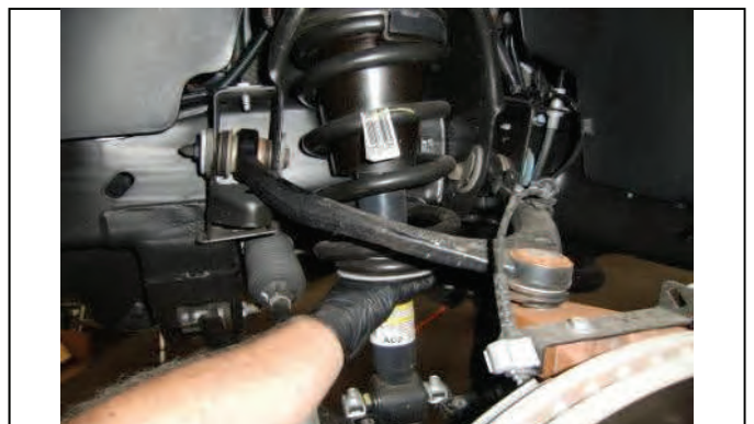
Remove entire strut assembly from vehicle.
