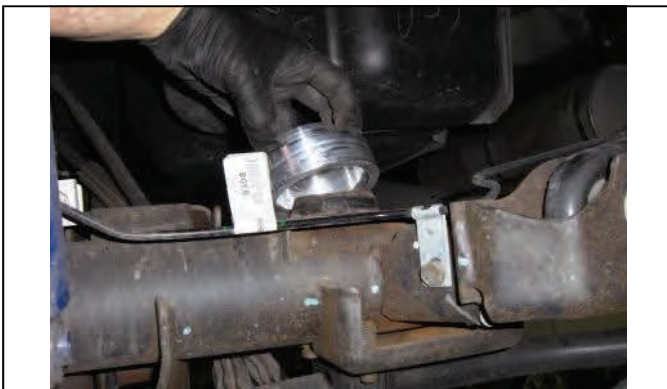
Place ReadyLIFT spacer on axle mount
