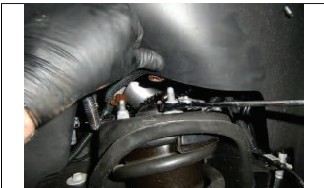
Remove upper strut mounting nuts
