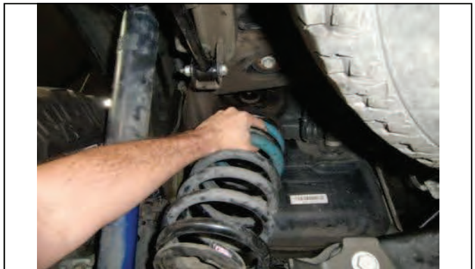
Carefully lower axle and remove coil springs and isolators
