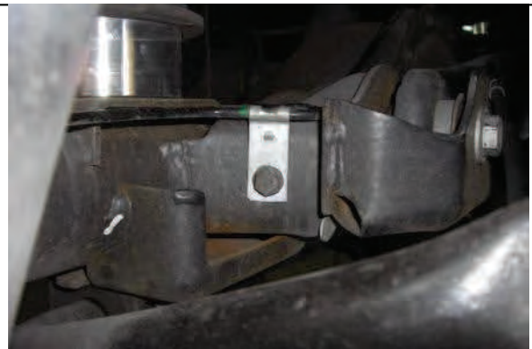
Unbolt dr/pass brake lines on axle
