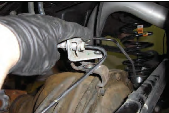
Disconnect brake lines at top of differential
