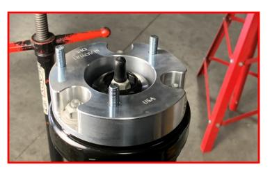
Using the supplied M10 nuts, install the completed strut assembly into the frame 180 degrees from the original orientation making sure that the offset of the top spacer is going in towards the frame and that the stamped word "OUT" on the spacer is going towards the outside of the vehicle. Do not tighten at this time.
