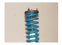
4. Take the stock strut assembly place into a vise, then use the external coil spring compressor to compress the spring enough to remove top nut. **WARNING: COIL SPRING IS UNDER EXTREME LOAD.** Remove the top nut and remove stock isolator mount, discard stock coil spring and shock.
