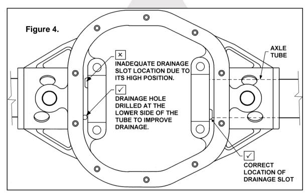
If drainage is inadequate or does not exist then a slot or hole should be cut into the housing on the lower side of the tube(s) to allow oil out of the axle tube area.
