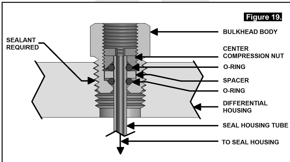
**NOTE :** Make sure the seal housing tube is all of the way into the center compression nut while you are tightening it.
