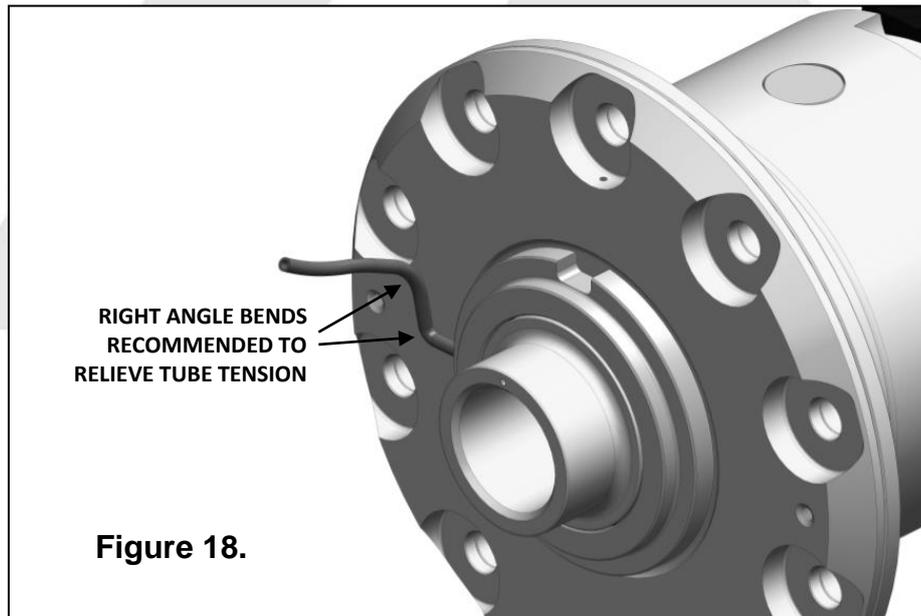
**NOTE :** Keep the tube away from the bearing cap or any other part of the differential casting as any contact due to vibration or shock may wear the tube and eventually cause a leak.
