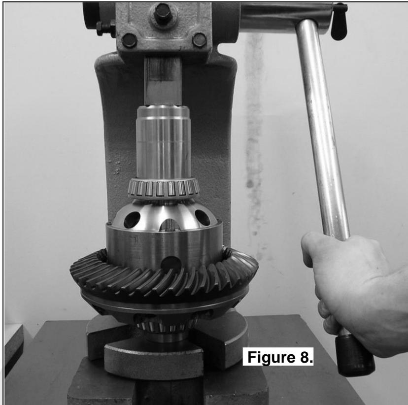
**NOTE :** The bearing on the flange case side can only be installed after the seal housing is assembled into the seal housing journal.
