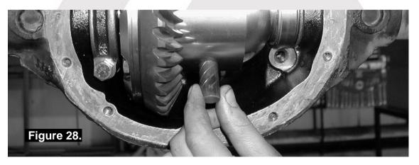
Rotate the differential until the 'C' clip access window is in full view.
