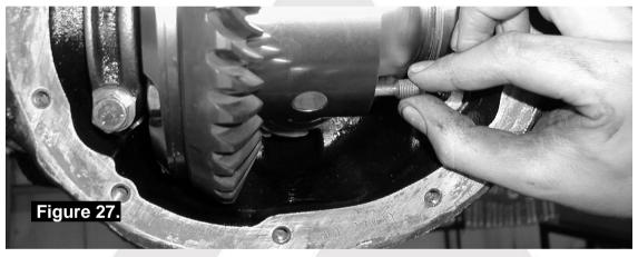
Completely remove the long cross shaft (Figure 28.)
