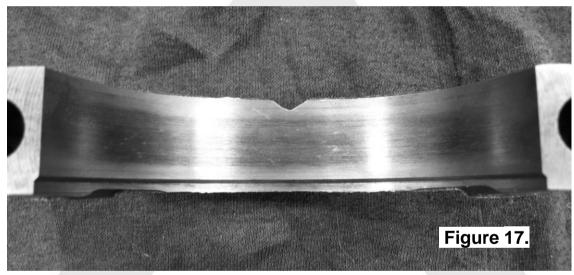
NOTE: Take time and double check when modifying the bearing cap, as they are custom fitted to the axle housing and cannot be replaced if damaged.
