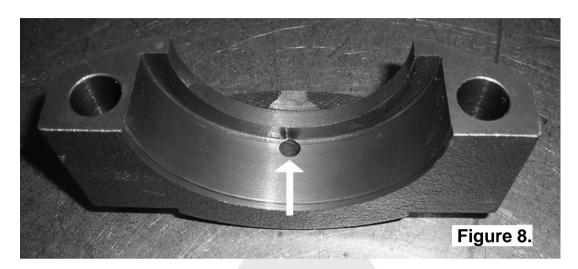
NOTE: Take time and double check when drilling, as bearing caps are custom fitted to the axle housing and cannot be replaced.
