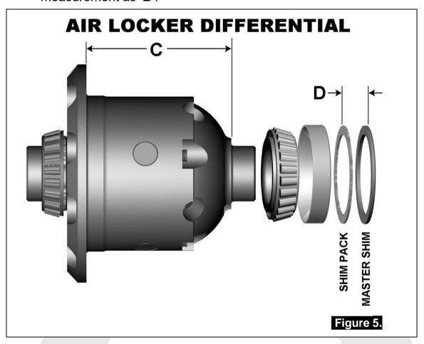
Measure the distance from the Air Locker bearing shoulder to the ring gear mounting face (shown as 'C' in Fig. 5.) and record this measurement as 'C'.
