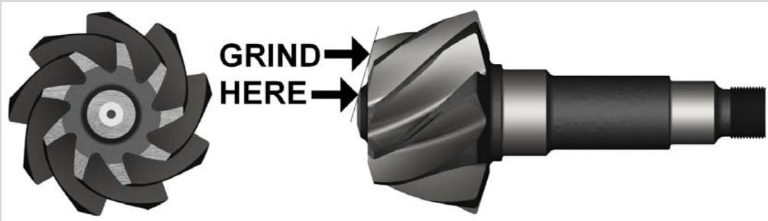
Clean all grinding particles from the pinion gear & differential housing after modifications.
