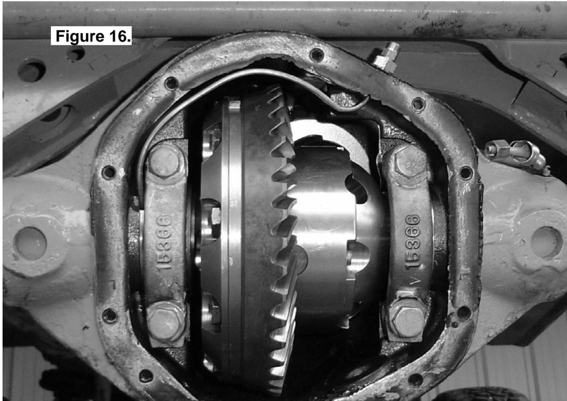
**NOTE :** It is also a good idea to keep the tube away from the bearing caps or any other part of the differential casting as any contact due to vibration or shock may wear the tube and eventually cause a leak.
