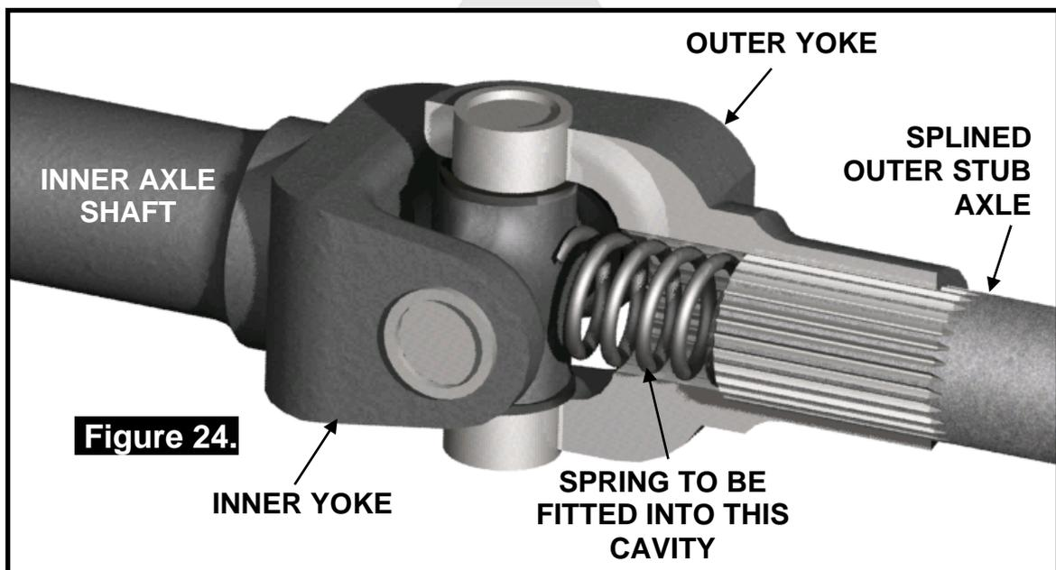
**NOTE :** When assembled, ensure that the spring maintains sufficient pressure on the axle to hold it firmly against the cross shaft of the differential while the vehicle is sitting on level ground.
