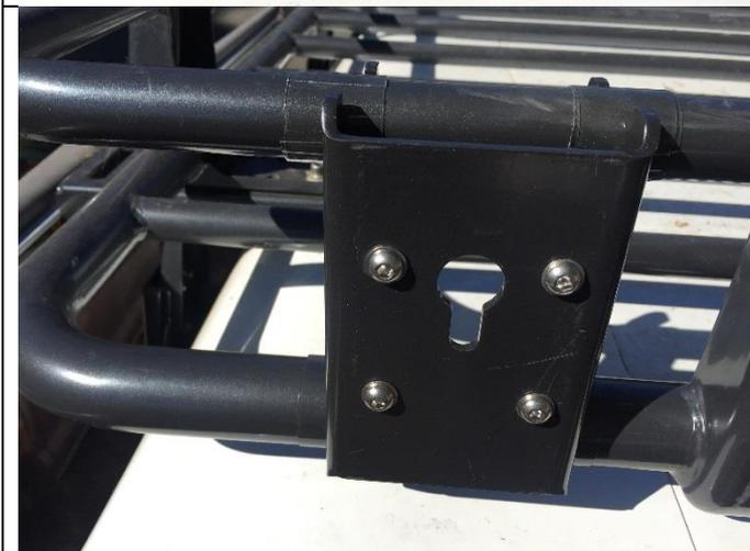
Place the outer bracket against the roof rack bars as shown.
