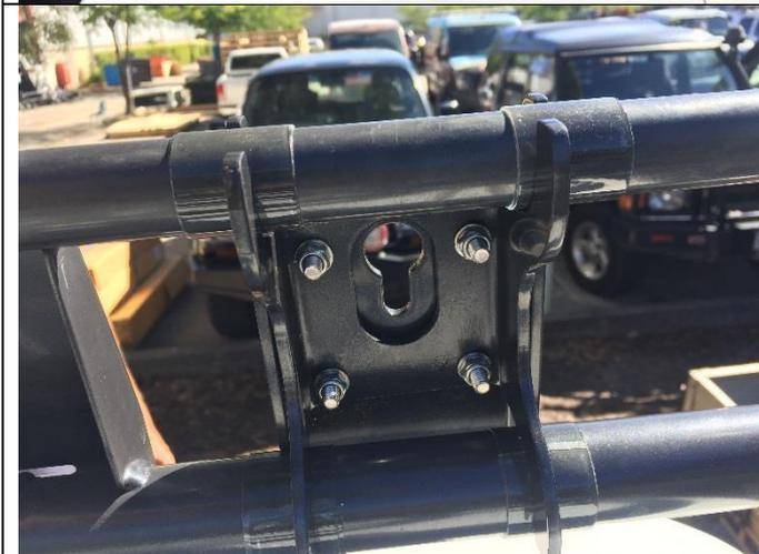
Place the inner bracket on the other side of the roof rack bars as shown.
