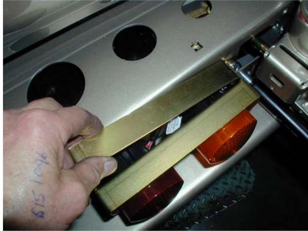
6. Fit M6 cage nuts to light mount cover bracket as shown below.
