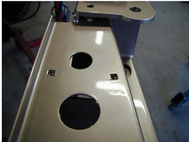
8. Fit M6 cage nuts (9 total) in square holes in top of bar as shown.
