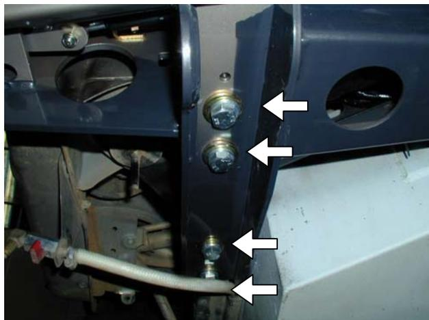
22. Fit eight **M14 x 40 x 1.5 bolts**, spring washers and large gold colored flat washers to underside of chassis rails. (LHS shown)
