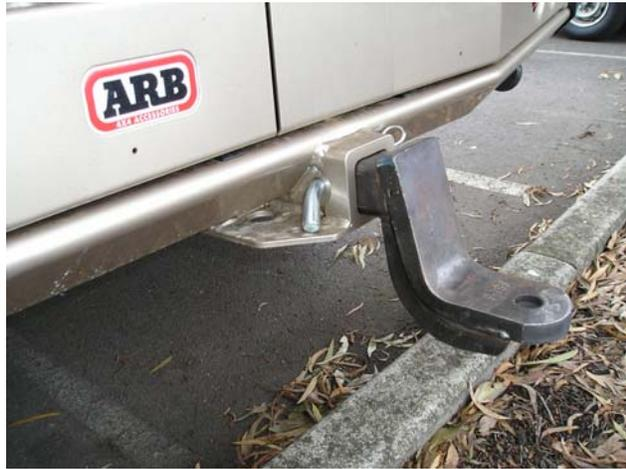
58. Fit gooseneck with pull pin and spring clip as shown.
