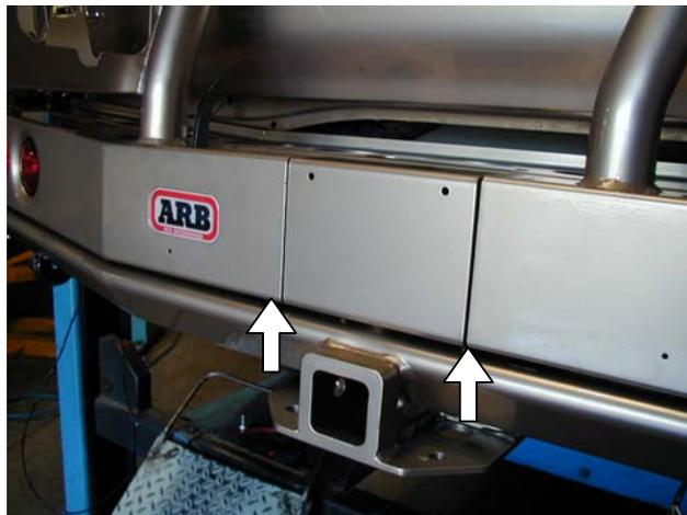
38. Align faces of centre cover panel with wheel carrier, jerry can carrier or cover panel and tighten securely.
