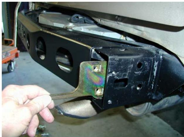
18. Fit **M12 x 1.75 cage nuts** to chassis side plates so that bracket assemblies are left and right handed, and insert into ends of chassis rails.
