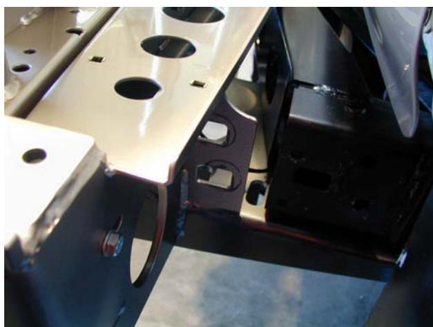
19. Slide bar onto rear of chassis leaving enough room to plug main loom into tail light assemblies on either side of vehicle.
