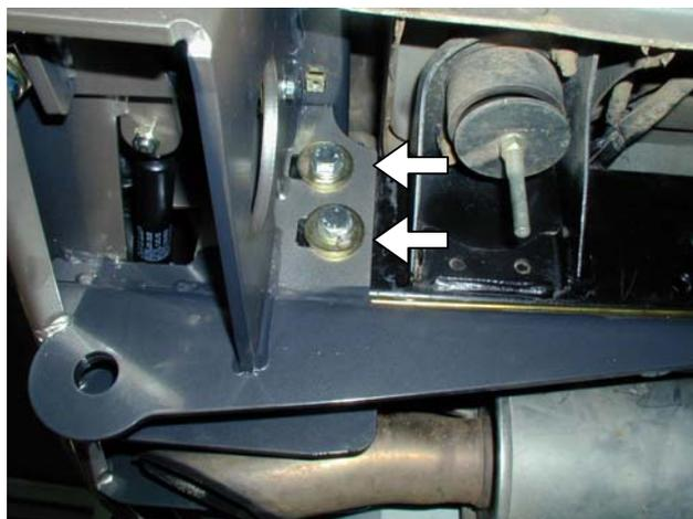
25. Fit two **M12 x 40 x 1.75 bolts**, large gold colored flat washers and spring washers into captive nut plates (installed previously – step16) on each side of vehicle.
