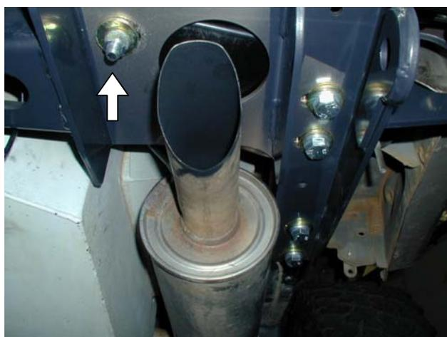
23. From inside chassis fit **M12 x 35 x 1.25 bolt** with extension plate (shown below) and large gold colored flat washer down through cross member and RHS chassis bracket.
