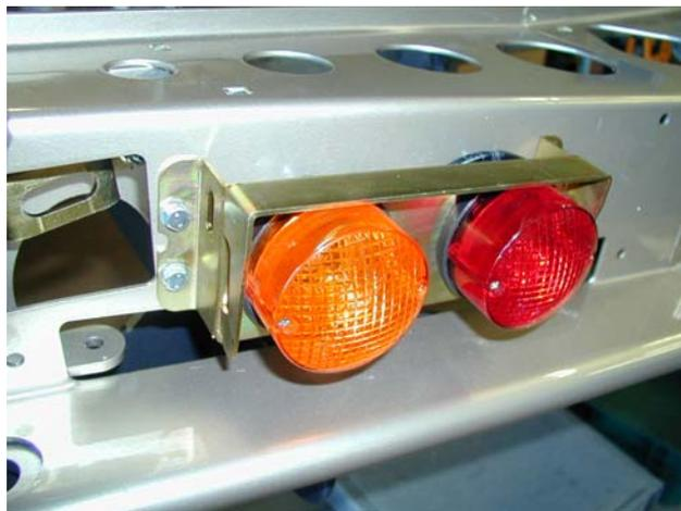
4. Fit light assemblies using M6 hardware. Finger tighten only.
