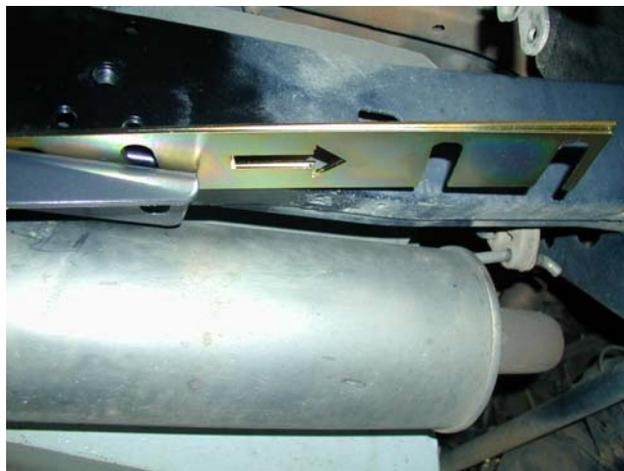
28. If not level, remove bolts from the side that is too high and insert a spacer plate between the chassis bracket and the chassis.
