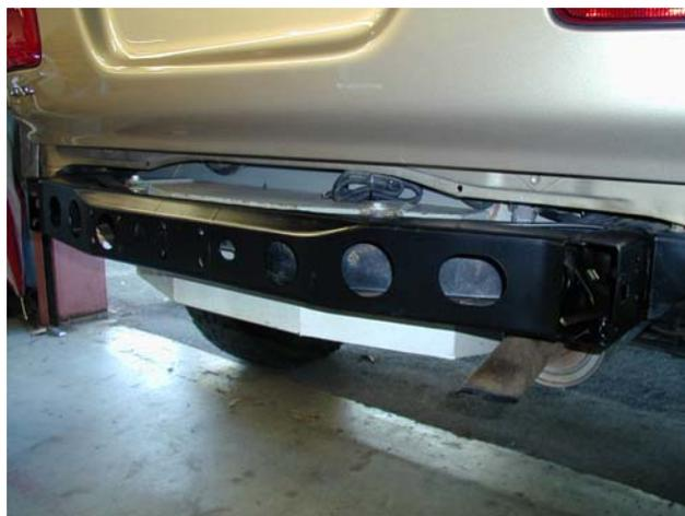
16. To fit Rear Bar to vehicle, remove bumper bar, mudflaps and tow bar (if fitted) from vehicle.
