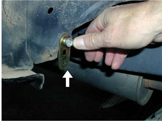
51. Using **M6 x 16 bolt**, flat washer and flange nut, fit mudflap mount plate to vehicle.
