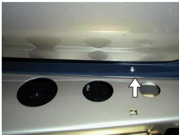
54. Using **M6 button head cap screws** fit top infill plate.
