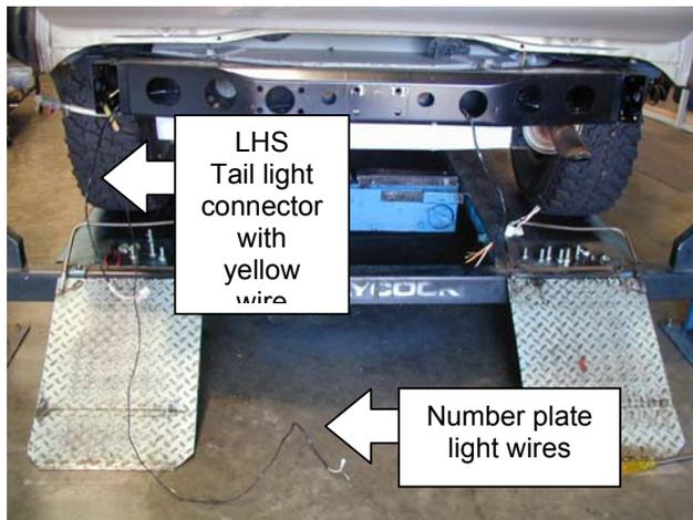
The loom is fitted with wiring for a number plate light.
