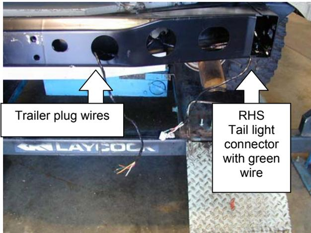
13. Exit tail light wires and trailer plug wires as shown.
