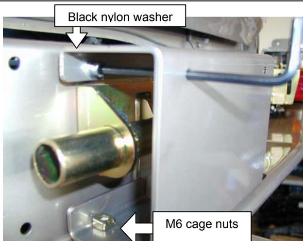
33. Place M6 cage nuts into lower section of centre cover panel.
