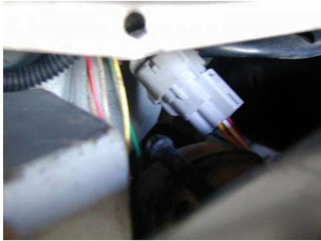
14. Make sure when plug is connected to vehicle that wire is cable tied well clear of muffler and exhaust components that may melt it.
