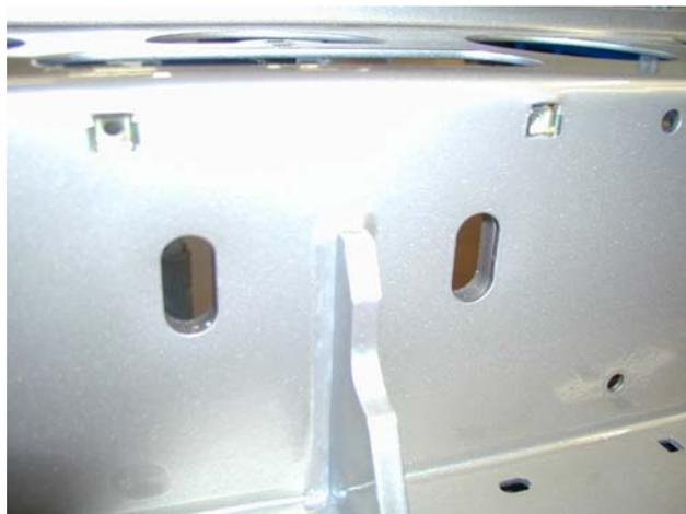
9. Fit M6 cage nuts (2 total) to front of bar.
