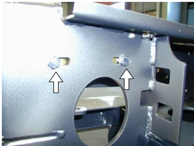
M8 bolts must fit in rear of bar for ease of adjustment later on.
