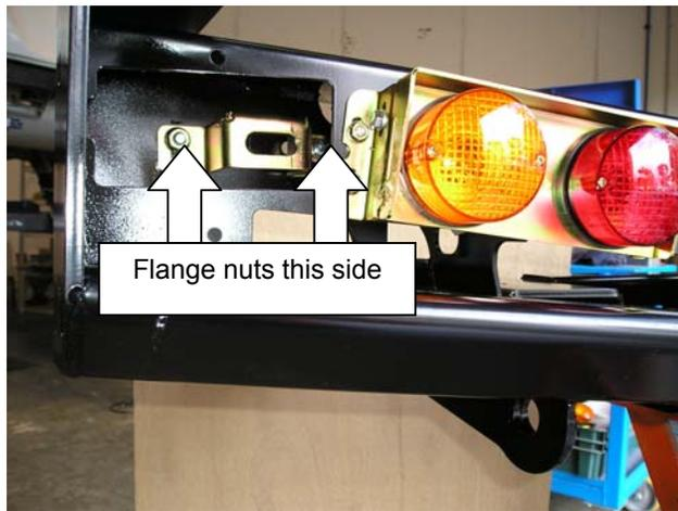
11. Fit locking pin brackets using two **M8 x 25 bolts**, flat washers and flange nuts. Finger tighten only.
