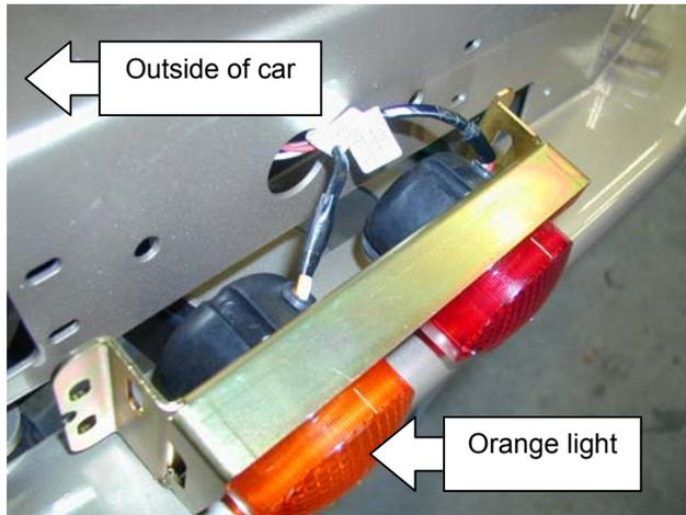
**When fitting light assemblies to bar, orange (indicator) lights must be to the outside as shown. The flange on the bracket should also be at the top.**
