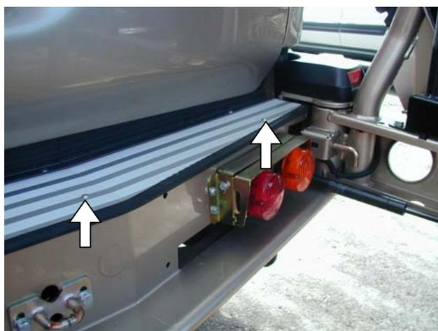
57. Using **M6 button head cap screws** fit aluminium step plate.
