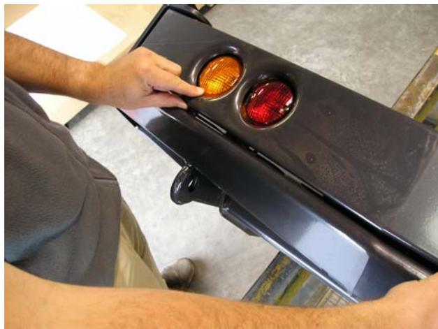
15. If a wheel carrier or jerry can carrier is not to be fitted a cover panel must be fitted.
