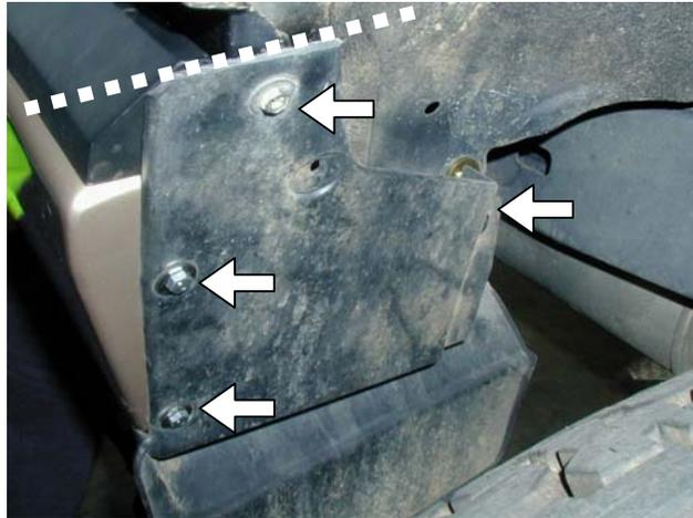
52. Fit mudflap top hole to original hole position of vehicle, then using M6 hardware, fit mudflap to rear bar end surrounds including lower end surround return as shown below.
