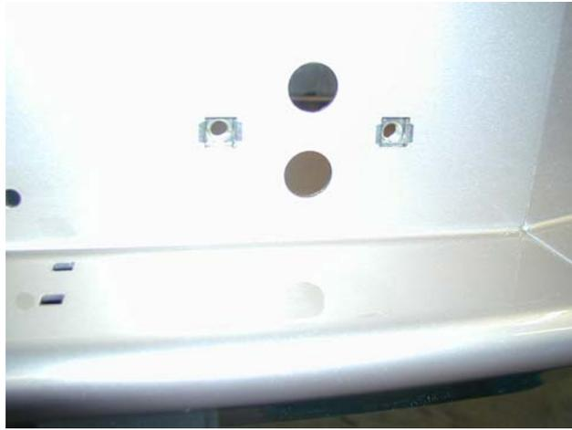
10. **If fitting a wheel carrier or jerry can carrier**, fit M8 cage nuts (supplied in wheel carrier fitting kit or jerry can carrier fitting kit) as shown.
