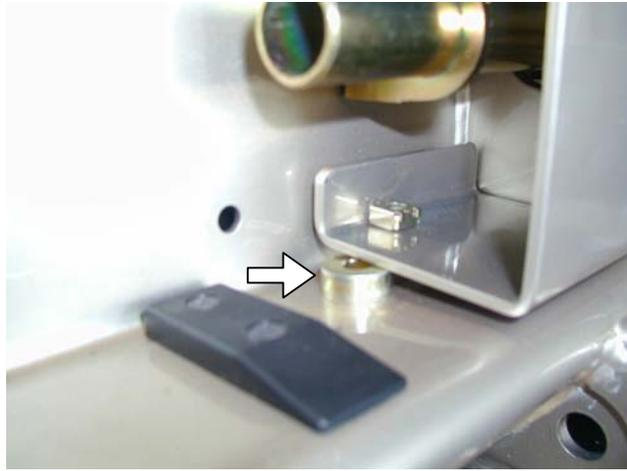
36. Place 8mm spacer between underside of centre cover panel and rear bar.
