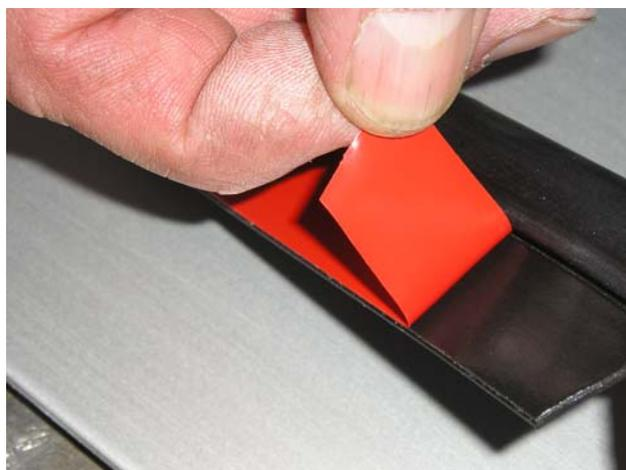
56. Carefully remove backing from tape on the rubber strip and fit to step plate working from the centre outwards. Make sure rubber strip hugs the front edge of the aluminium step plate.
