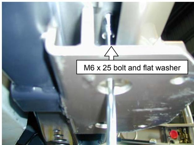
37. From underneath rear bar pass two **M6 x 25 bolts** and flat washers through the aligned parts and finger tighten.
