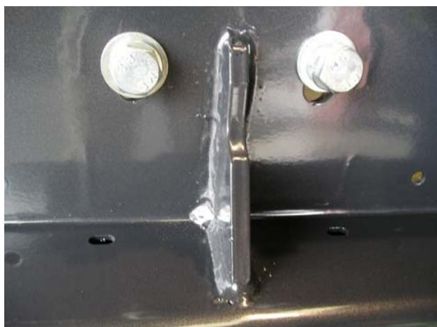
21. Fit two **M12 x 40 x 1.25 bolts**, spring washers and flat washers as shown into centre mounting bracket. (Finger tighten only.)
