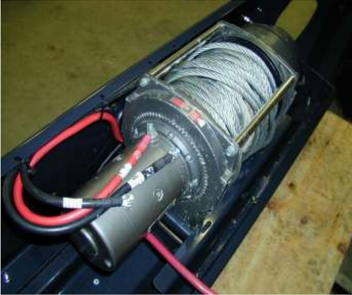
26. Install the winch and roller fairlead using bolts, nuts and spring washers supplied by Warn, and the 25 x 11.5 x 1.6mm flat washers supplied in the bolt kit. Refer to Warn installation instructions for correct procedure. Adjust winch in slots until the winch is centralized in the bull bar.
