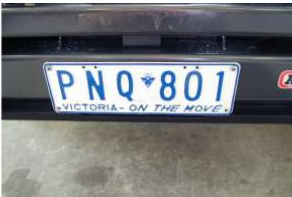
20. Bolt the number plate through the top holes using M6 X 16mm bolts and M6 flange nuts. If desired double sided tape can be used down the sides of the number plate.
