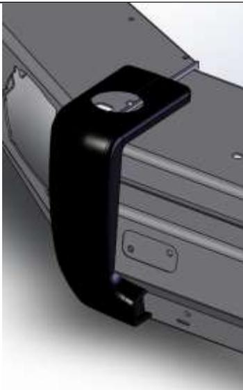
9. Insert the side buffers through the holes and fix using the M6 flange nuts. (Do not over tighten). (RH shown).
