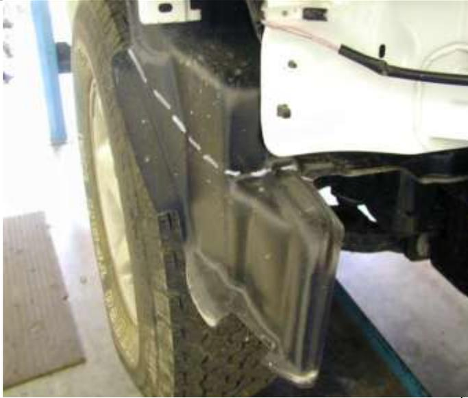
2. Using sharp scissors or a cutting blade, cut the plastic inner guard as per line shown in the photo. (RH shown).
