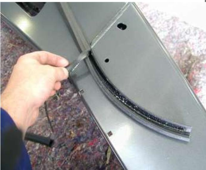
31. The rubber extrusion contains a support section to assist in the moulding. Remove this section by tearing at one end. Discard this section.
