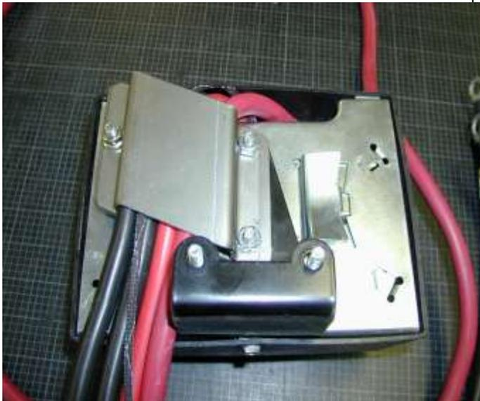
22. Undo the screws on the side of the control box, remove the top cover and replace the three short leads with the longer ones supplied in the fitting kit.
