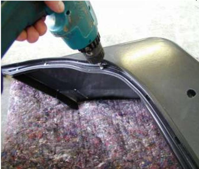
34. Using a Phillips head screw driver or cordless drill with a Phillips head tip fix the extrusions to the top of the wings using the self-tapping screws.
