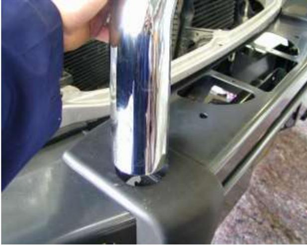
16. Push the top Sahara tube through the hole in the buffer and fasten using the M12 x 40mm bolts, washers and spring washers.
