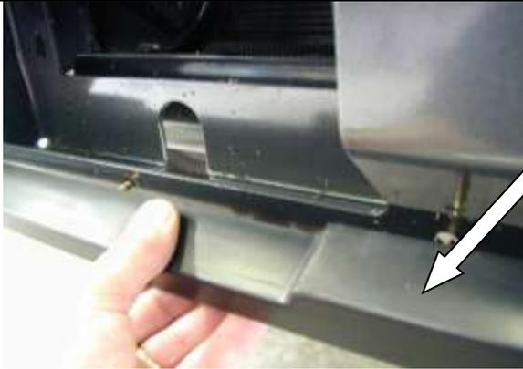
8. Position the lower buffer on the winch bumper and assemble using the M6 flange nuts. (Do not over tighten).
