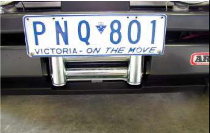
28. Peel off one side of the double sided tape and adhere to the top rear side of the number plate. Note: Clean the adhering surfaces before applying tape with an alcohol solvent.
