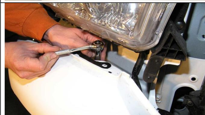
11. Remove screws retaining bumper located under headlamp area.
