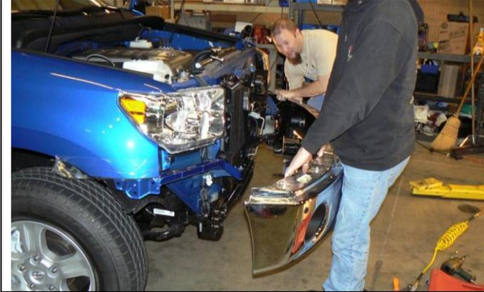
19. Remove crash bar and lower bumper assembly and set aside, retain flange nuts for reuse.
