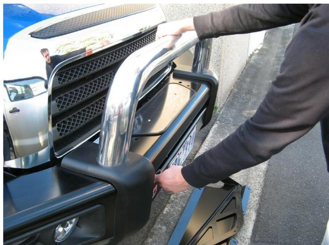
65. Test the operation of the frame tilt assembly
