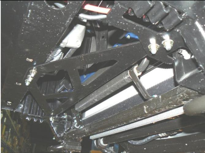
76. Bolt the bar to the mounts using M12 bolts. Large flat washers and spring washers. Centralise the bar to the front of the vehicle.
