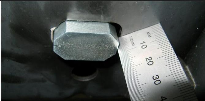
78. Tighten up the mount brackets fasteners. Start with the tow hook bolts, then M10 flange nuts to chassis studs.
