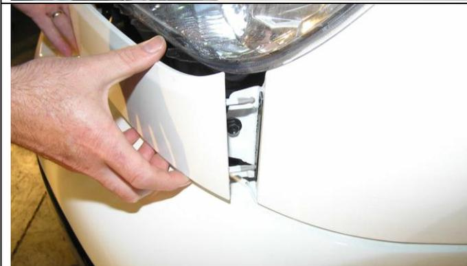
10. Carefully prise the trim pieces free by pulling them forward and twisting to release plugs out of retaining sockets.
