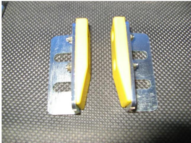
63. Fit a urethane buffer pad to each of the right angle brackets using M4x16 csk head screws and M4 nyloc nuts, to create a pair of RH and LH assemblies as shown.
