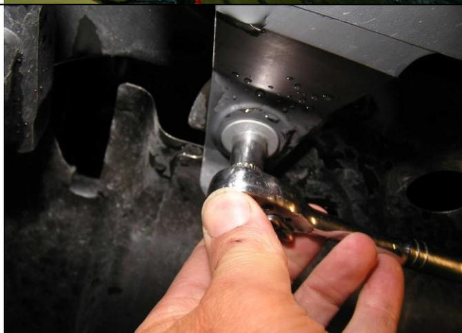
3. Remove lower bumper retaining screws.
