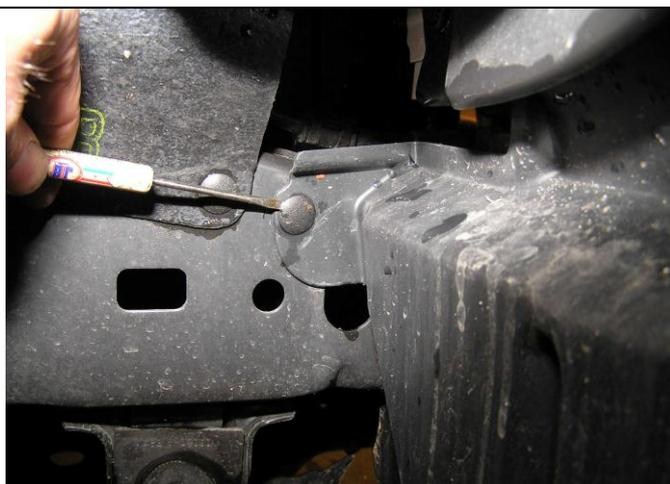
6. Prise out lower fender liner plastic push in plugs. Remove lower fender liner completely, they will not be reused.
