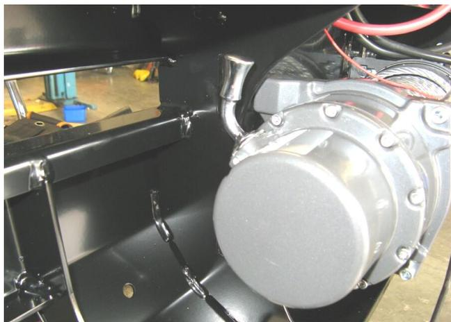
36. Position the winch with the mount face facing upward on an adjustable table or similar and with the assistance of another person lower the bulbar over the winch. The winch handle should be in the LHS of the bull bar for smaller winches than 12-15000lb winches which are on the opposite side as they spool in the opposite direction. The cable must always spool off the bottom of the winch.
