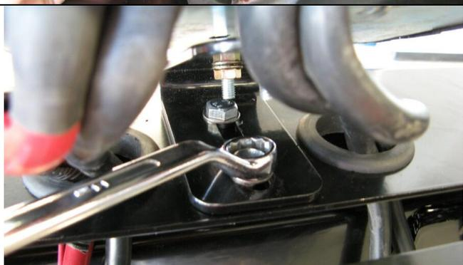
31. Using M8 fasteners fit control box mounting bracket to pan
