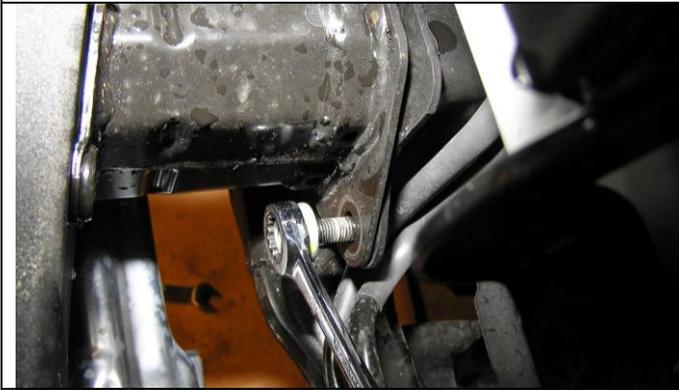
18. Undo crash bar mounts from chassis flange.
