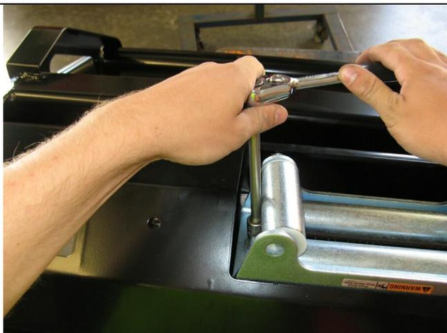
37. Fit the roller fair lead, pull only the end of the cable through and adjust the position of winch then bolt up securely. Use the 1 ½" long bolts in the top and 1 ¾" in the lower set through the RFL.
