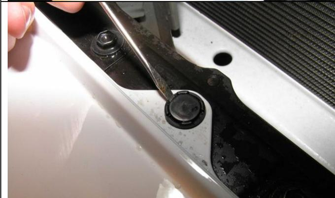
12. Remove plugs securing upper bumper tabs.
