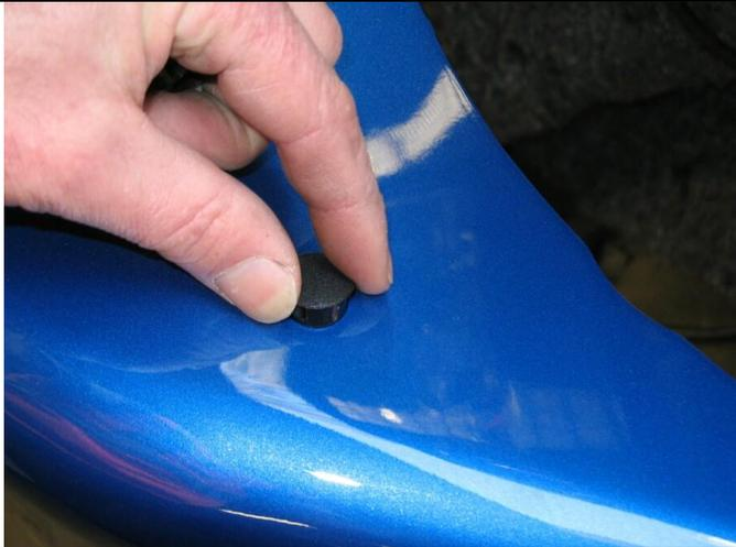
80. Unless fitting CB aerials, fit blanking plugs in provided holes in the top of the wings.
