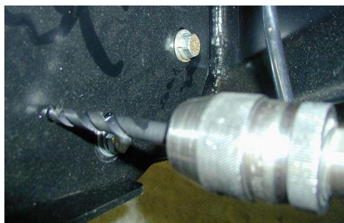
64. Using the M10 pilot hole in mount brackets, drill pinning hole through uprights of bull bar. Fit M10 SEMS bolt and flange nut, do up tight to recommended torque.
