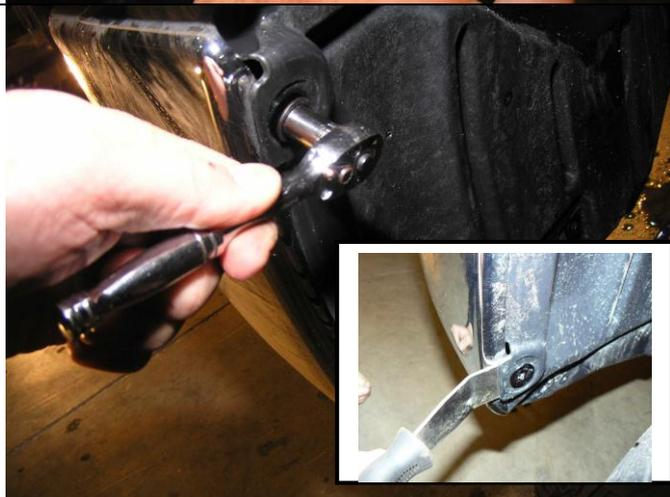
4. Remove all lower fender liner retaining screws to bumper.
