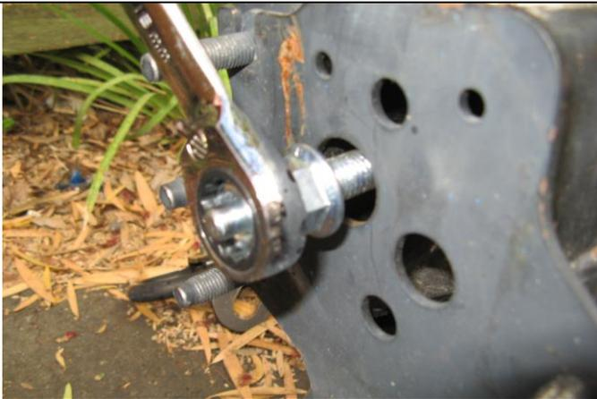
24. Install the chassis stud by fitting 2 nuts to the end of the stud and tightening until thread bottoms out.
