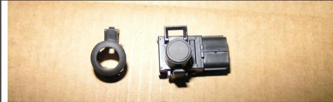
20. If parking sensors fitted and are to be reused, remove from bumper. Also retain loom tails and set aside.
