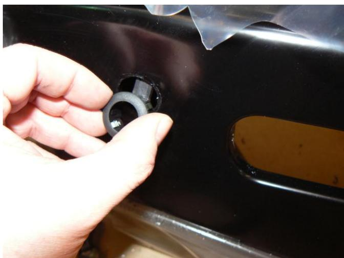
44. Once sensor hole is cut and sensor has been trial fitted, paint the raw metal edges to prevent corrosion.
