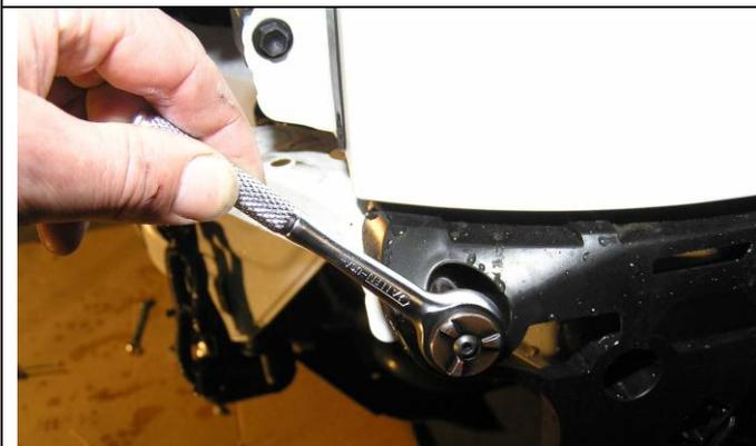
21. Remove bumper cover retaining brackets from the fenders.
