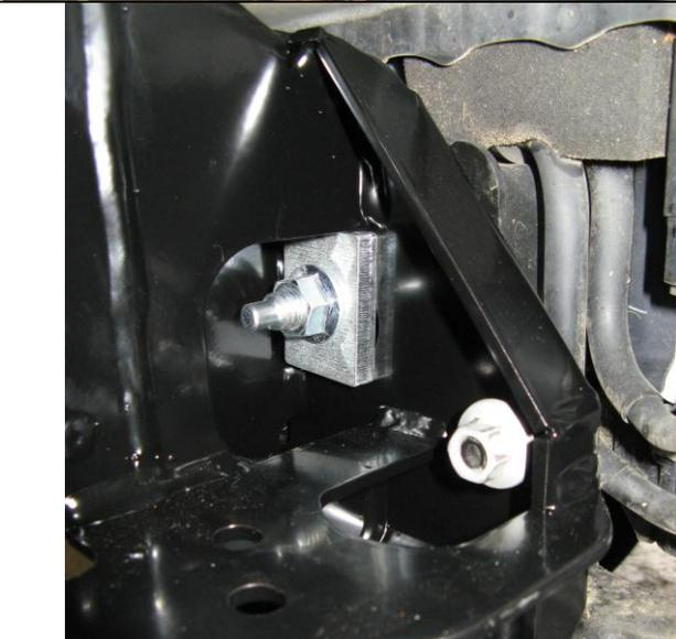
26. Loosely fit the mounting brackets to the chassis securing with the 8mm packers and flange nuts.
