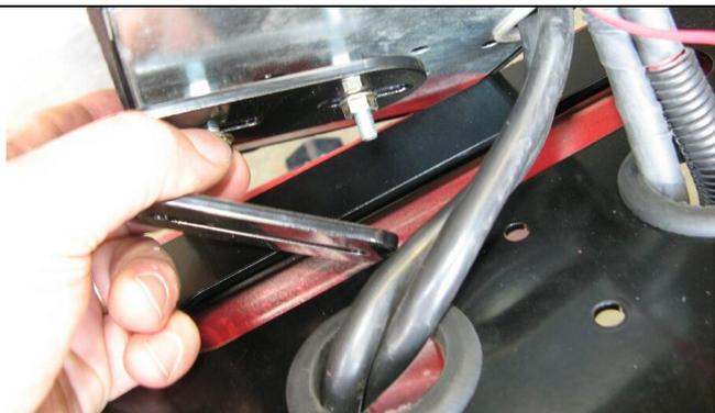
29. Fit large grommets to holes in top pan
