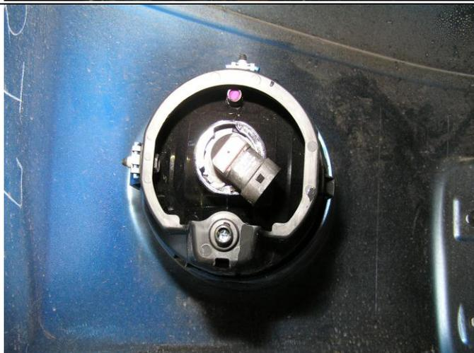
7. If OE fog lights and/or parking sensors fitted in bumper, undo electrical connections.
