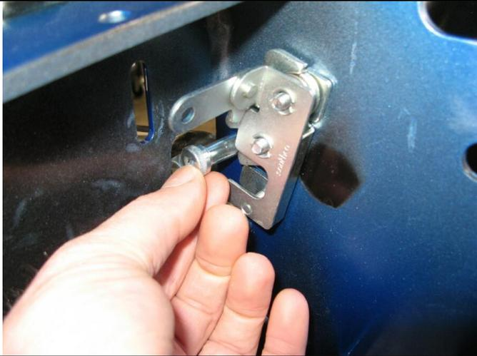
62. Fit the striker pin to the **RHS** hinge plate and secure with 5/16"UNC nut and spring washer as shown and tighten to 22Nm or 16lbft
