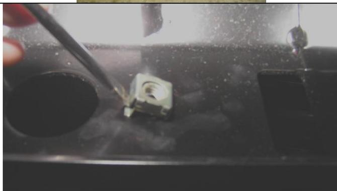
53. In lower inside face of pan, fit M8 cage nuts for stone tray in four positions as shown.
