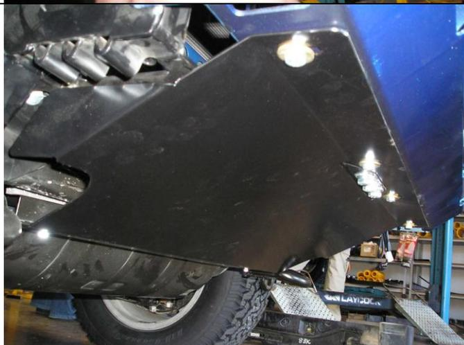
79. Fit stone tray using 4 x M8 bolts and washer sets at front and 2 x M8 bolts, washers and into fitted M8 cage nuts at two locations into existing sump guard front section as shown.
