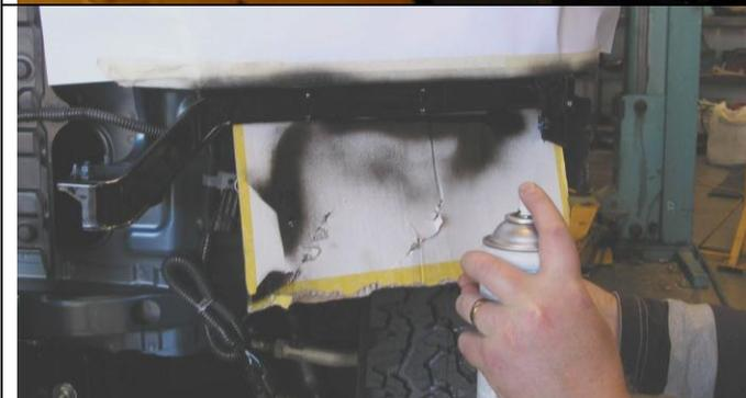
22. Mask up and spray paint the exposed metal trim area black satin, from the wheel arch right around to the inboard headlamp area as shown, both sides of the vehicle.
