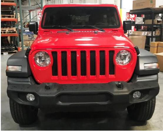
1. To fit the bull bar to the vehicle, the plastic bumper and associated hardware must be removed from the vehicle.
