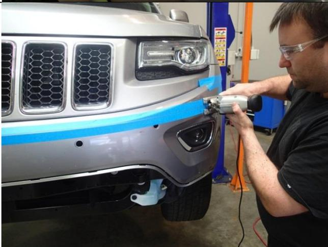
24. Using a jigsaw carefully cut along the lines marked above removing the lower section of the bumper.
