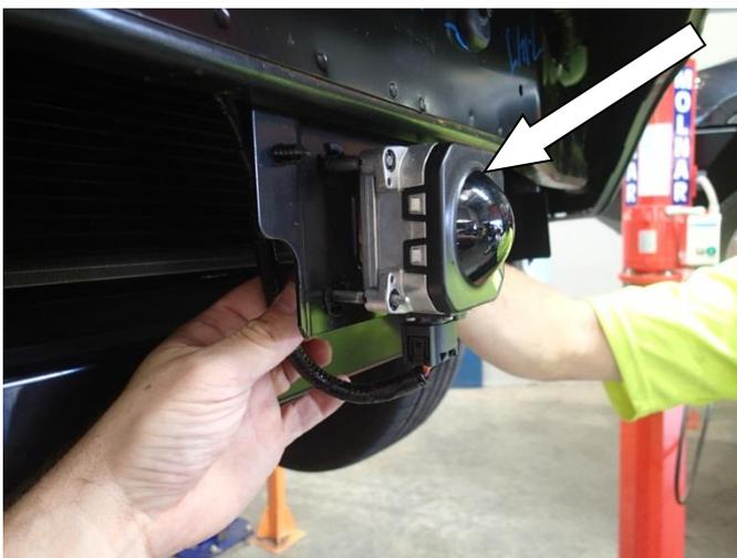
**IF RADAR FITTED REFER TO STEPS 10-12, IF NO RADAR IS FITTED MOVE STRAIGHT TO STEP 13**
