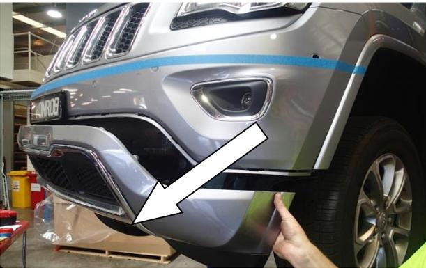
5. Undo the clips on each side of the vehicle and remove the lower section of the bumper.
