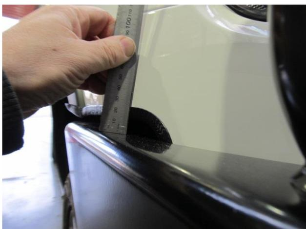
76. Adjust the bar so that it is central to the vehicle and has an even gap of between 8-14mm between the rear edge of the bar and the vehicles bumper.
