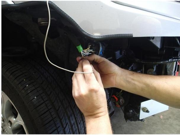
33. On each side of the vehicle identify the wire for the indicators and the clearance lamps using the chart below.
