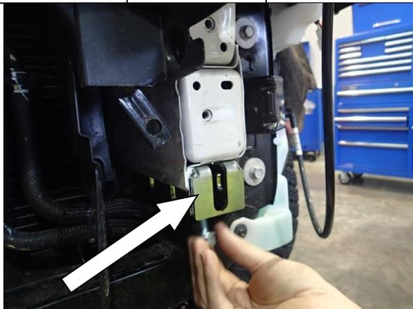
36. Attach the chassis mount braces to the bottom face of the chassis rails using 2 x M10 SEMS bolts in each side. Leave loose at this stage.
