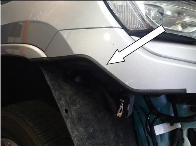
26. Attach pinch weld to each side of the vehicle as shown.
