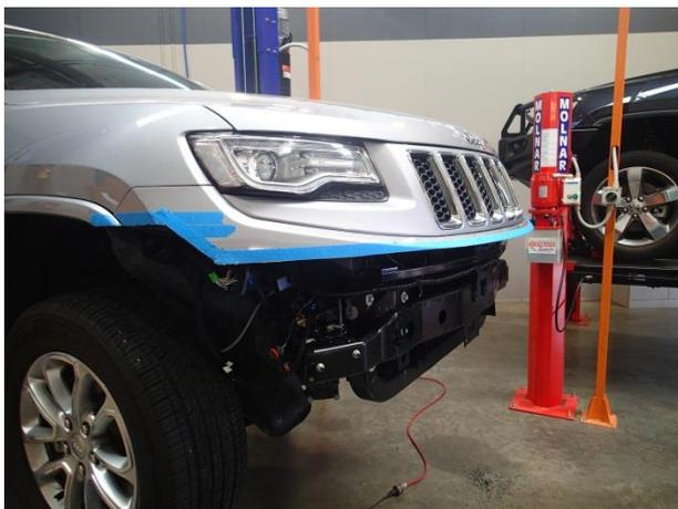
25. Using sandpaper or a file, remove any sharp edges.
