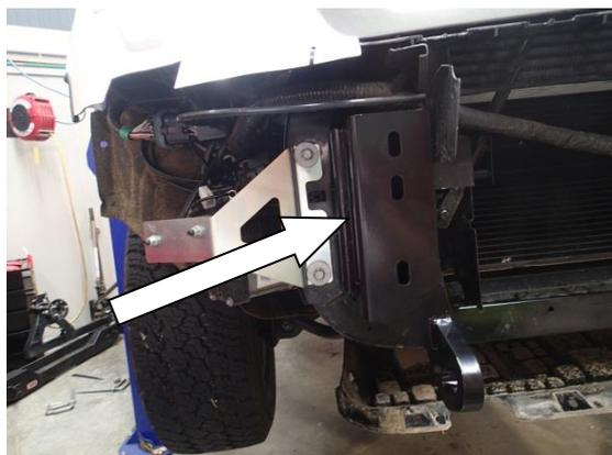
38. Attach the mount brackets to the chassis ends using 2 x M8 x 25 hex bolts, M8 spring washers and flat washers in each side. Leave loose at this stage.
