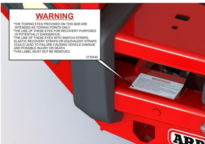
91. Place the tow warning label onto the top surface of the lower pan as shown.
