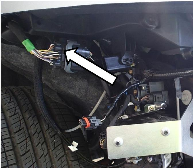
32. On each side of the vehicle, locate the wiring loom connectors.
