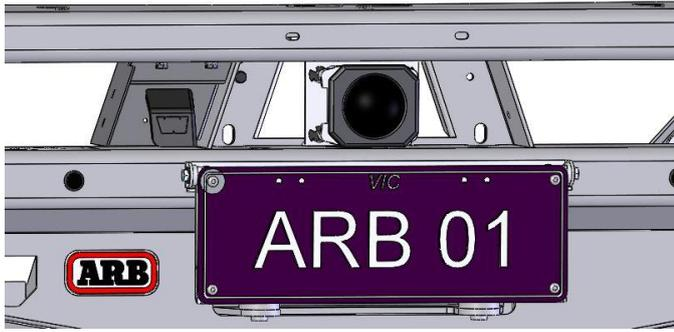
71. If fitting a winch and a radar sensor attach the folding license plate bracket supplied in kit 3540050 to the lower pan using M6 SS button head screws, M6 SS flat washers and M6 flange nuts.
