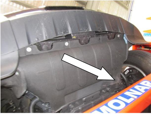
1. Remove the 3 screws and 1 plug holding the stone shield to the cross beam and discard.
