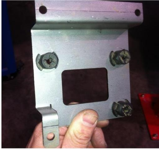
57. Fit the plastic lugs removed about to the radar sensor bracket as shown by inserting the lugs and turning  $\frac{1}{4}$  turn clockwise.
