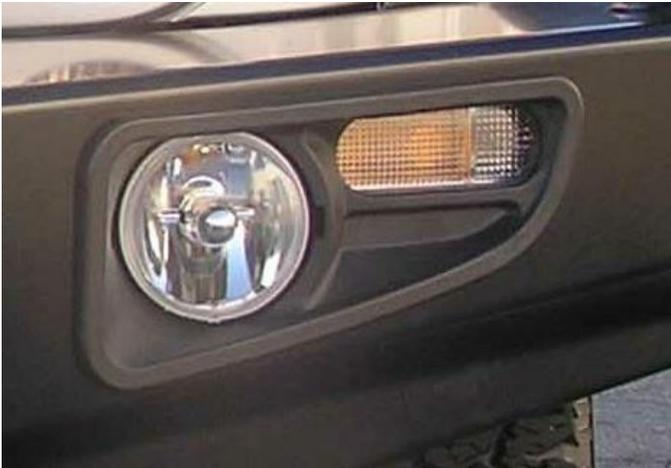
56. Assemble and install combination light surrounds (p/n 3163015) as per instructions no. 3786421 supplied with surround kit. Note: Optional fog lamps can be installed at this point as per fitting instruction no. 3783315 supplied with fog lamp kit no. 6821201.
