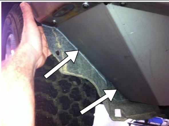
83. On each side of the vehicle, hold the inner guard against the wing and under wing panel.
