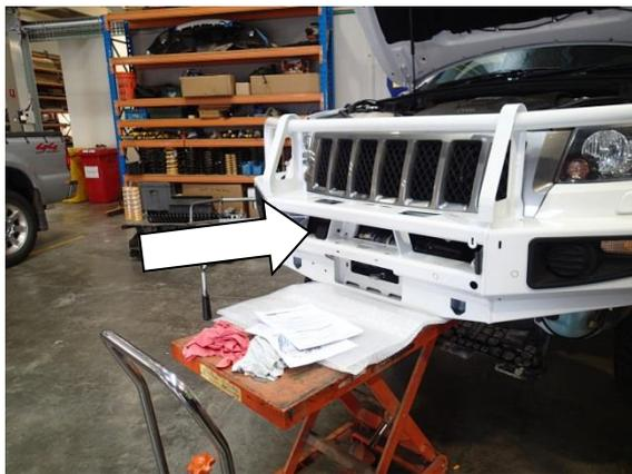
74. With the assistance of another person or a lifting device, lift the bar onto the car so that the mount faces of the bar align with the faces of the mount brackets.
