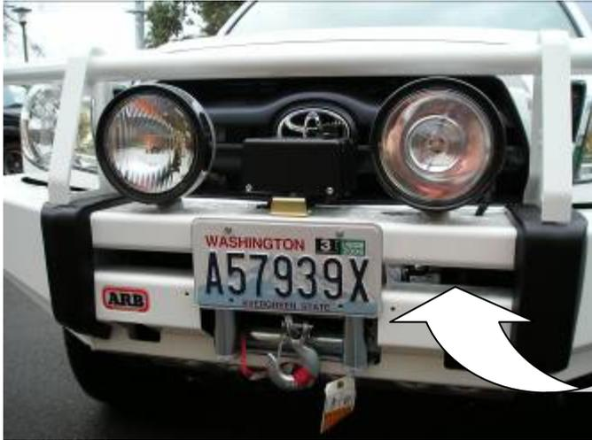
41. Fit number plate to number plate bracket using M6 hardware.
