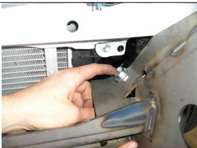
7. Fit M12 x 1.25P X 35mm (fine thread) bolt with 12mm flat washer through top rearward bracket passing through body mount.
