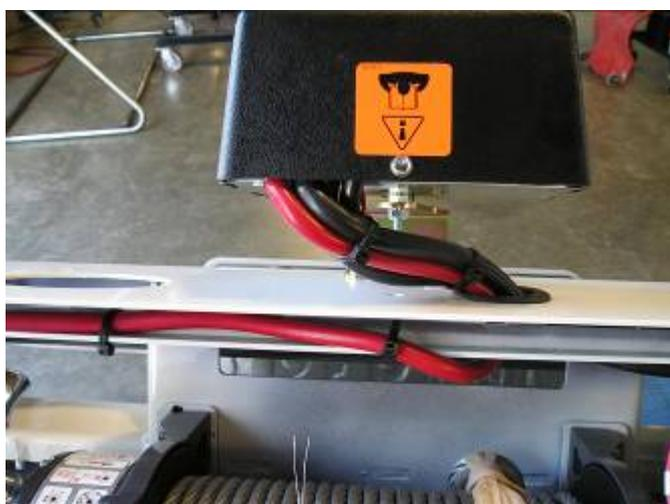
31. Fit control box to control box bracket and pass cables through rubber grommet.
