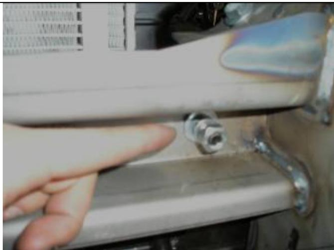
6. Fit 10mm x 1.25mm nuts ( fine thread) spring washers and flat washers ( from bull bar bolt kit ) to both the centre studs. **See Photo:**
