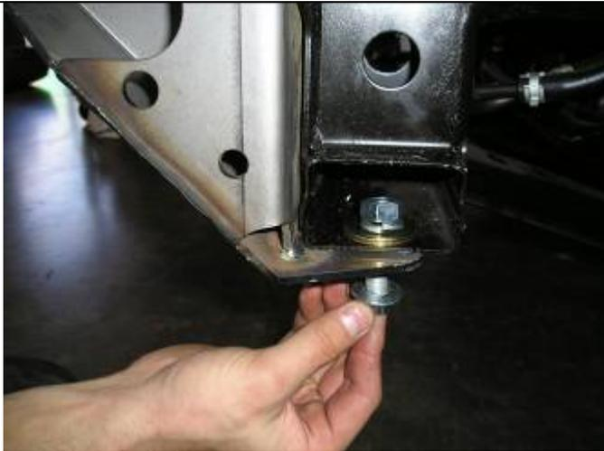
9. Secure lower fixing point by passing through lower bracket in a upward motion, using M12 bolt, 12mm flat washer and secure from the top using large gold coloured 12mm flat washer, 12mm spring washer and M12 nut ( fine thread ) to each side of vehicle. When all bolts are fitted, tighten securely.
