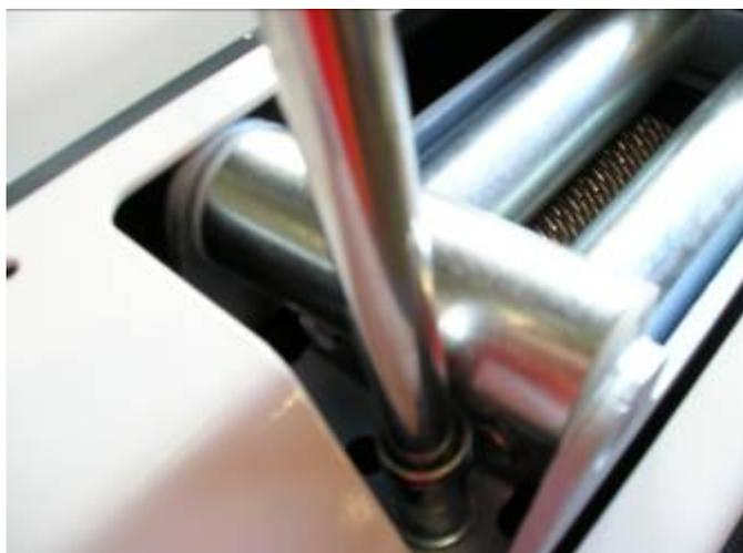
29. When all bolts are fitted and tighten, refit vertical roller pins back into roller fairlead and refit circlips.
