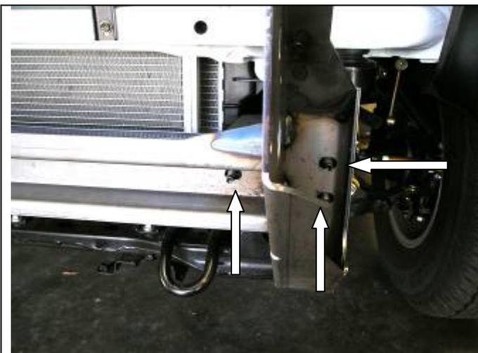
4. Fit bracket mounting assembly to front of vehicle using the 6 x 10mm studs to locate on.
