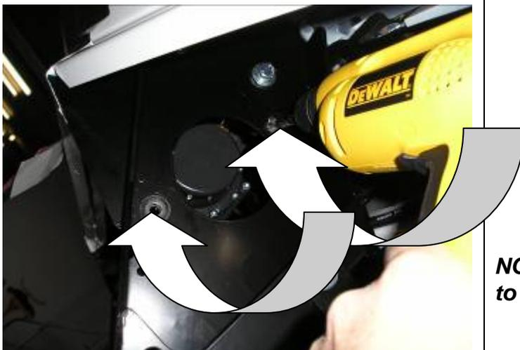
36. Finally, using the existing 2 holes as a template. Drill through using a M10 drill bit and secure using the balance of the 10mm hardware.
