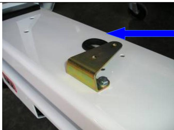
22. Bolt control box bracket to top of bar using 8mm hardware.
