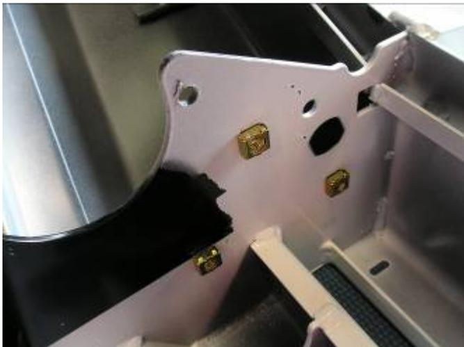
13. Fit M10 caged nuts to the inside of mounting surface of bull bar.
