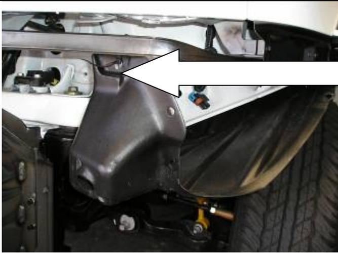
12. Cable tie under guard plastic moulding up to vehicle front pan.
