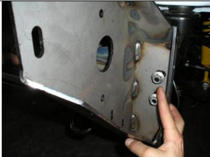
5. Fit original 10mm nuts to the outside fixing points . **See Photo:**
