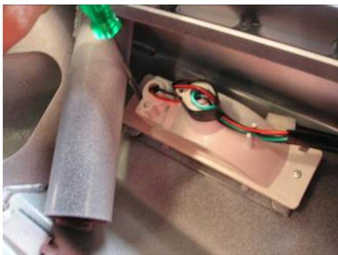
15. Align indicator/parker light above white nylon plugs and secure to bull bar using self tapping screws.
