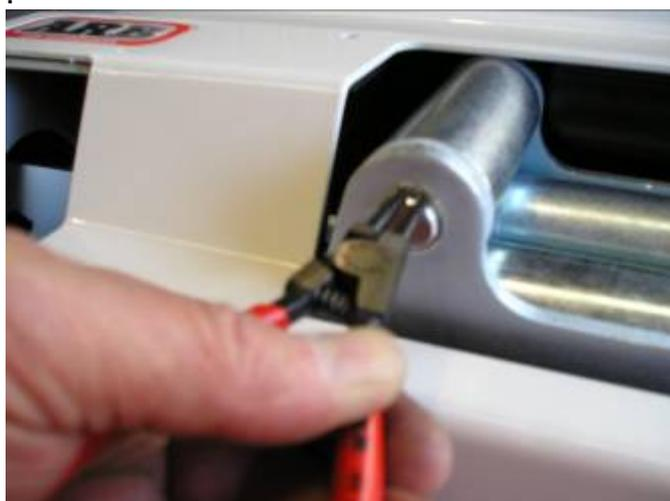
27. Position the roller fairlead, and remove the circlips from the lower of the vertical rollers and push the pins up to give access to the lower bolts.
