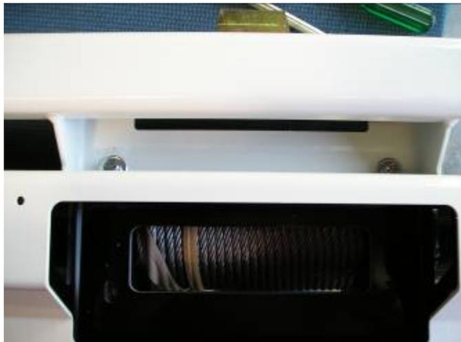
25. Place the winch on a table with the feet facing up and using an assistant; carefully lift the bull bar on top of the winch.
