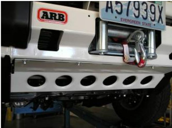
38. Fit splash pan to lower flange of bull bar using M6 x 20mm bolts, 6mm spring washers and 6mm large flat washers.
