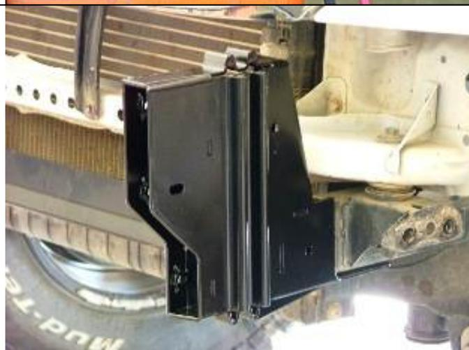
17. Fit 3 x M10 cage nuts to inner face of both impact absorbers.
