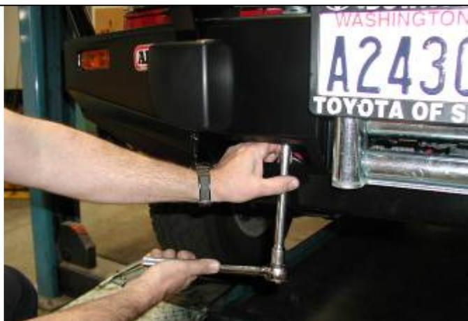
35. If driving lights are to be fitted, use extension bar with ratchet,  $\frac{3}{4}$ " long reach socket to tighten from cutout in centre pan
