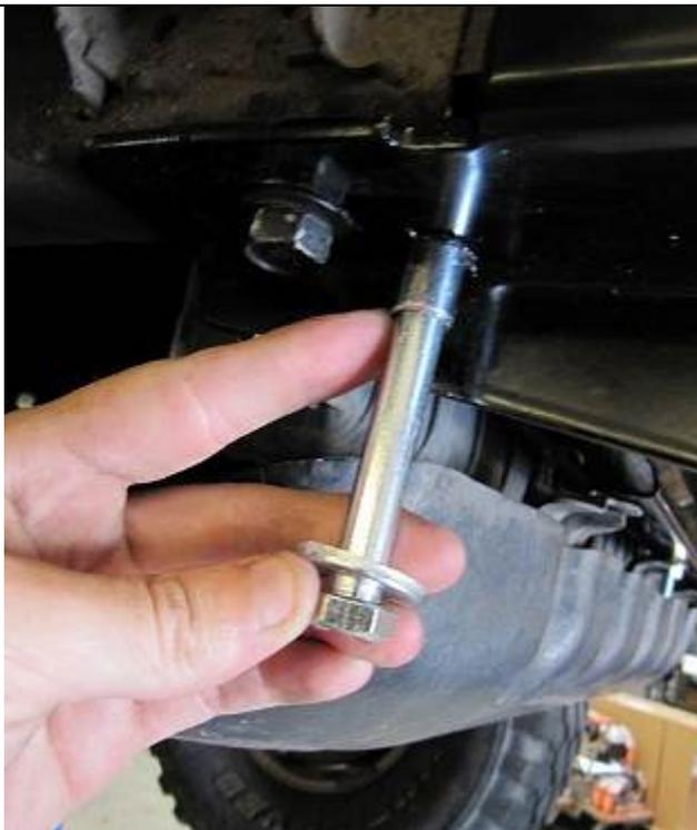
23. Fit M10 x 110 bolts, with M10 flat washers and Dia 13 OD spacer tubes up through pinning holes and secure with 2 x M10 flat washers and M10 nyloc nuts. ***Tighten fully to specified torque***
