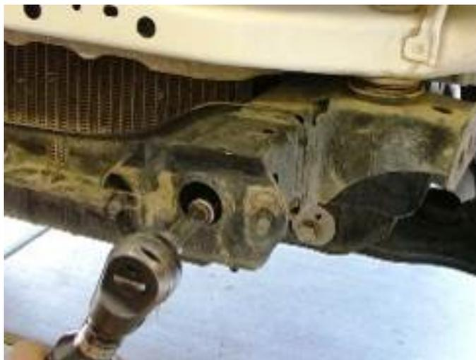
1. Remove bumper bar, tie down rings, and tow hook from the vehicle.
