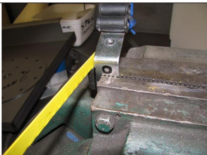
50. Modify the clamp plates for the power steering pipes by cutting off the flange as shown then drilling a Dia 8.5 hole 8mm from the bend as shown
