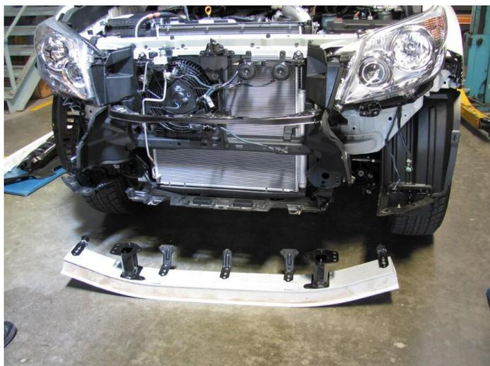
30. Remove reinforcing beam at mounts to chassis by undoing the M10 fine thread bolts. Set beam aside, it will not be reused
