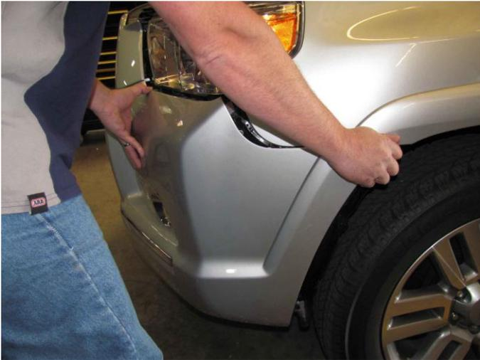
18. Carefully, and ideally with the aid of a friend, unclip each outer of the bumper at the guard as shown and remove bumper.
