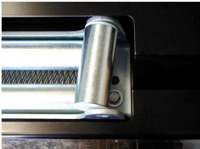
60. Remove the cir clips from the bottom of the vertical rollers of the fairlead and push the pin upwards. Push the vertical rollers inwards on the lower edges as shown and using two 3/8" x 1 3/4" bolts M10 flat and spring washers, attach the lower section of the roller fairlead to the bull bar and winch.
