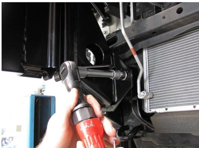
46. Fit impact absorbers to chassis ends using ***fine thread M10 x 1.25P x 30 bolt*** and washer sets supplied, note that the brackets are handed, slide them towards the centre of the vehicle on the adjustment slots ***do not do up tight***
