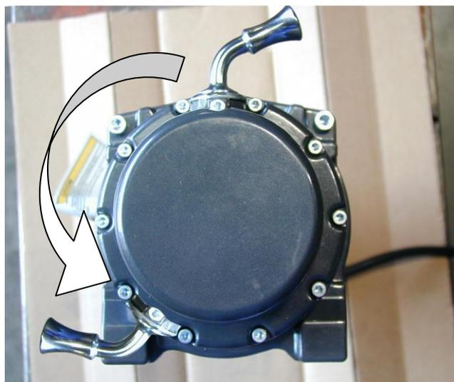
57. Remove the cap head screws retaining the gearbox to the winch drum. Carefully lift the gearbox a small amount (5 mm ) and rotate 144 degrees counter clockwise (four hole spacings) and re-fit the cap screws . This places the winch handle in the correct orientation.
