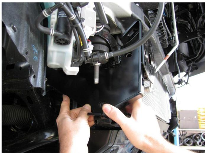
38. When the RHS side brace are fitted in position as shown, insert **fine thread M12 x1.25P x 30 bolt** and washer sets into lowest hole position to chassis. There is an existing captive nut in chassis, **but do not do up tight.**
