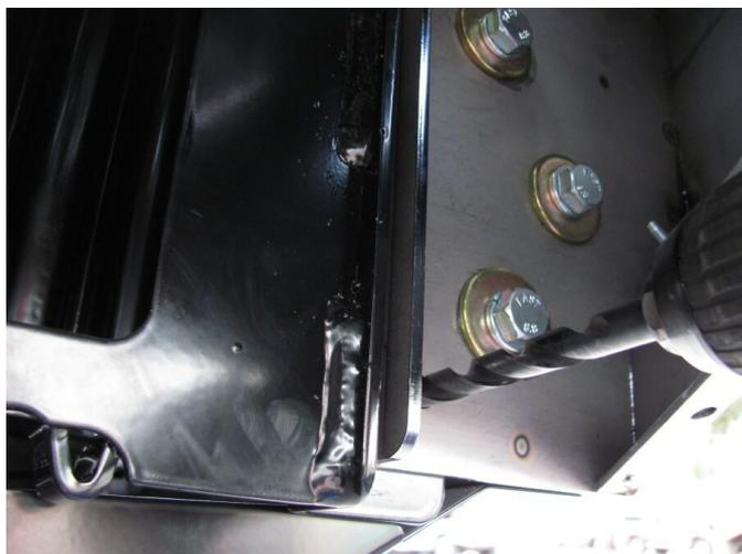
73. Using an electric drill and a Dia10.0 mm drill bit, drill two pinning bolt holes through the bull bar upright each side using the holes in the mount bracket flanges as a guide. One hole is located in the lower lug of the mount face and one up above the welded nuts. Use access through the light surround opening for the top hole.
