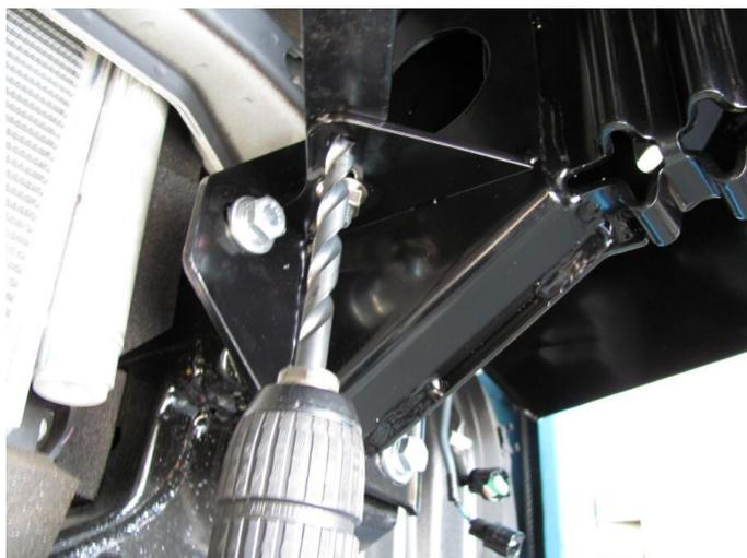
76. Using a Dia10mm drill bit, drill and pin the straps at the adjustment end using the pilot hole as a guide, as shown (note strap fits above the gusset as shown).
