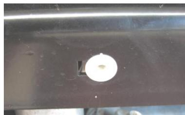
88. If winch fitted, position the licence plate as shown fastening top picture using lower holes. If winch not fitted use the top row of holes, licence plate is positioned lower and covers RFL opening in front of bull bar, lower picture.
