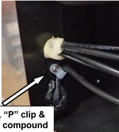
Insert new thermistor
