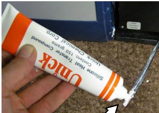
Apply heat transfer paste
