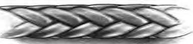
Rope exhibits fiber-set from compression. A slight sheen is visible. This is not a permanent characteristic and can be eliminated by flexing the rope.
