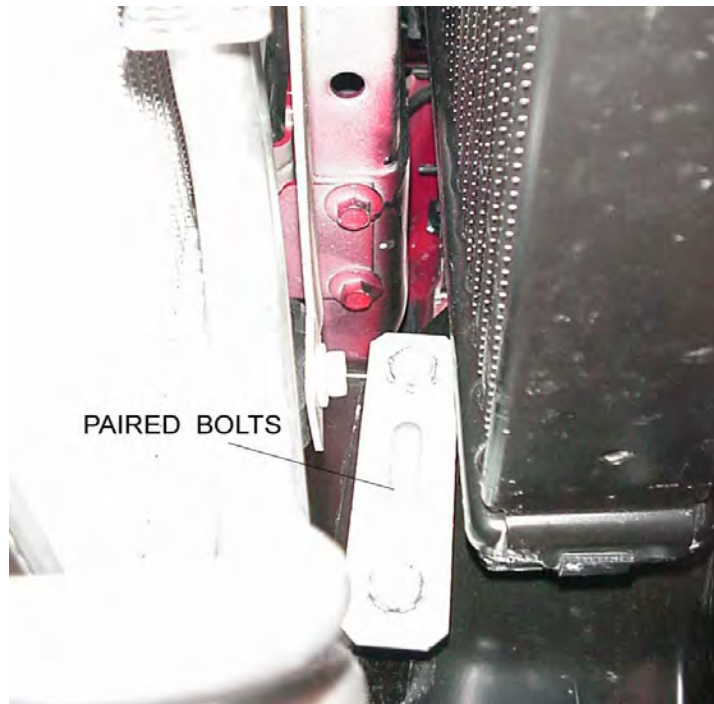
Figure F: Bolts attaching bumper brackets to frame (viewed from center of vehicle, looking outward)
