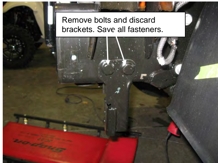
Figure H: Left (driver side) Blocker beam bracket.
