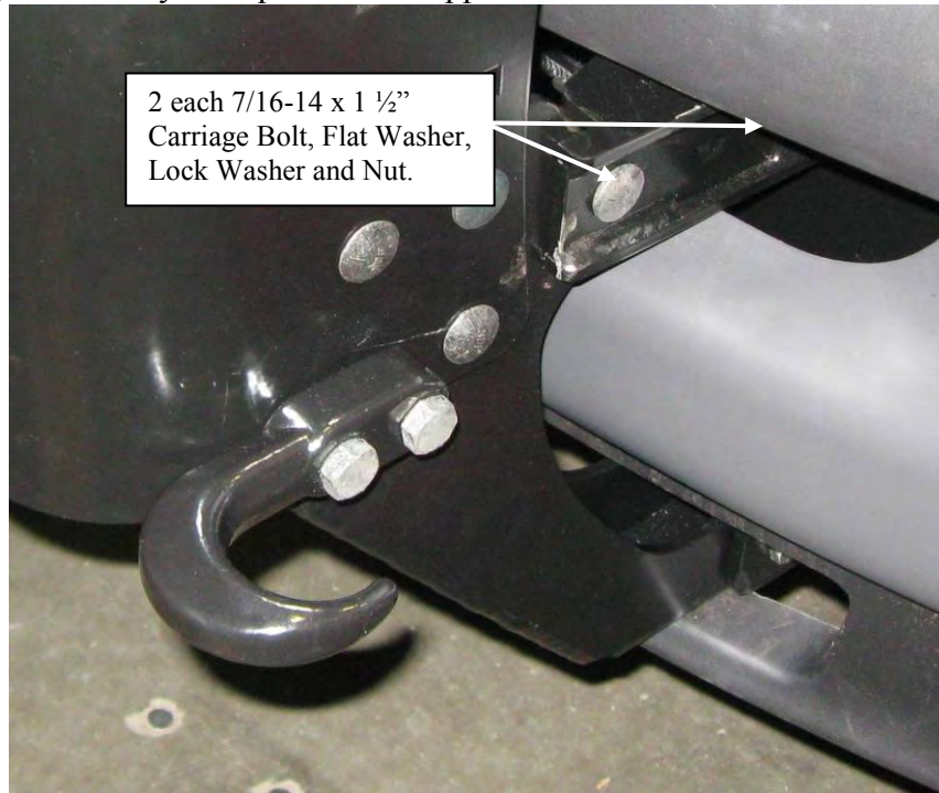
Figure 6: Large Frame Carrier: Top Carriage Bolt Positions.
