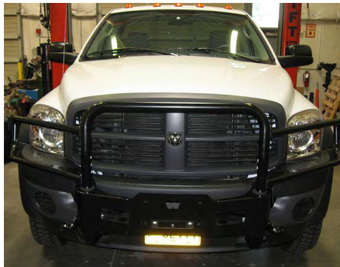
Figure 13: Finished kit (Winch Not Included) (Shown with optional center tube and headlight guards)
