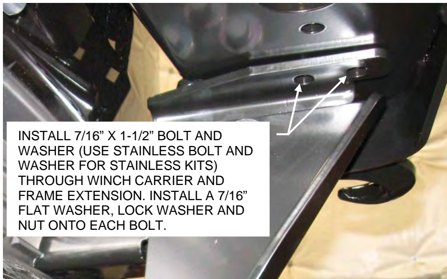
Figure 8: Winch Carrier to Frame Extension bolts
