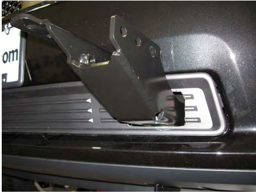
Figure 5: Installation of Frame Extension Bracket, Driver's Side Shown
