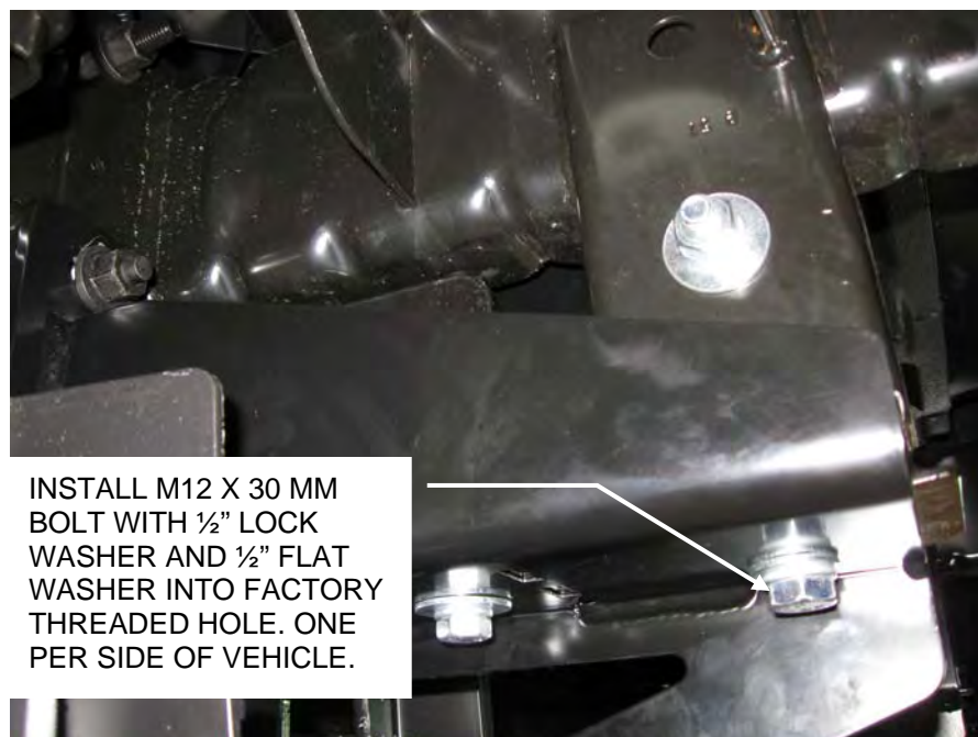
Figure 3: Installation of bottom frame bolt, M12 x 30mm
