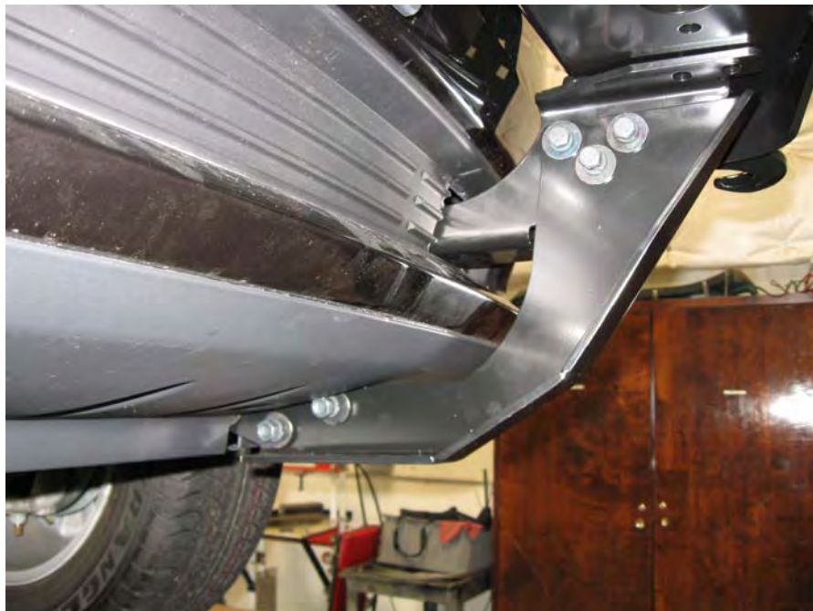
Figure 9: Driver's Side View. Lower Frame Bracket Installation
