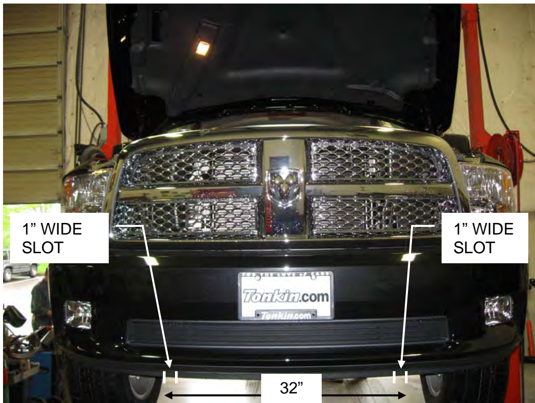
Figure H, Cut 1" wide access slots into factory air dam, 32" outside to outside of slot.
