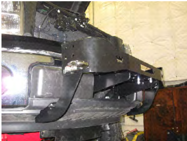
Figure 8. Tow Hook Installation.
