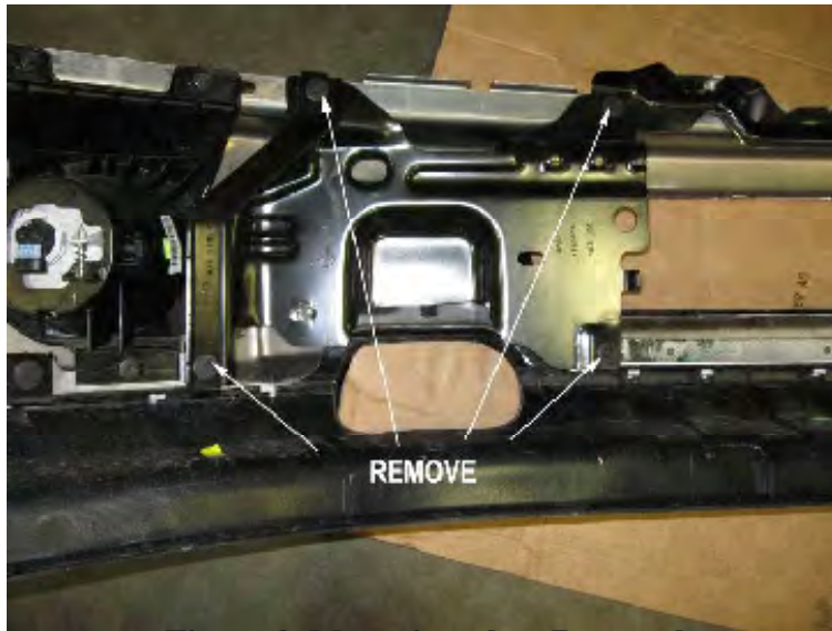
Figure 3. Mounting plate Removal
