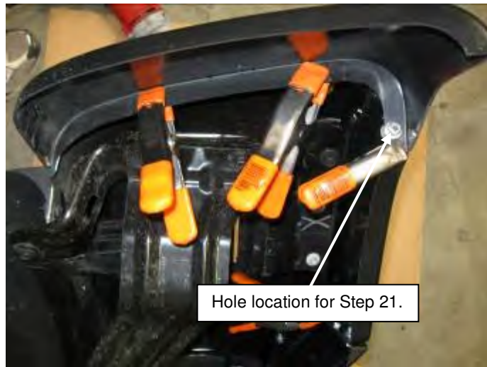
Figure 12: End Cap Installation. (Bumper flange holes not shown)
