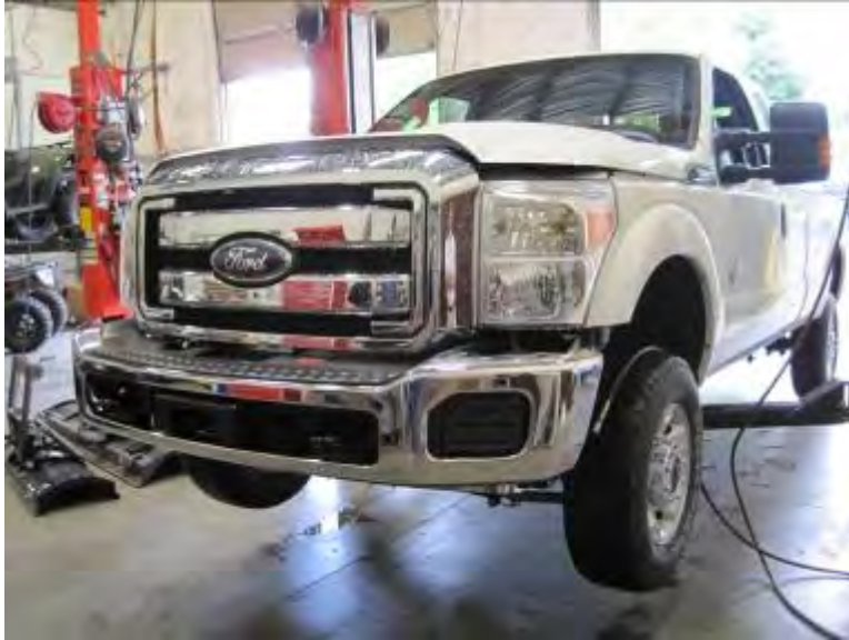
Figure 21: Bumper installed and leveled.
