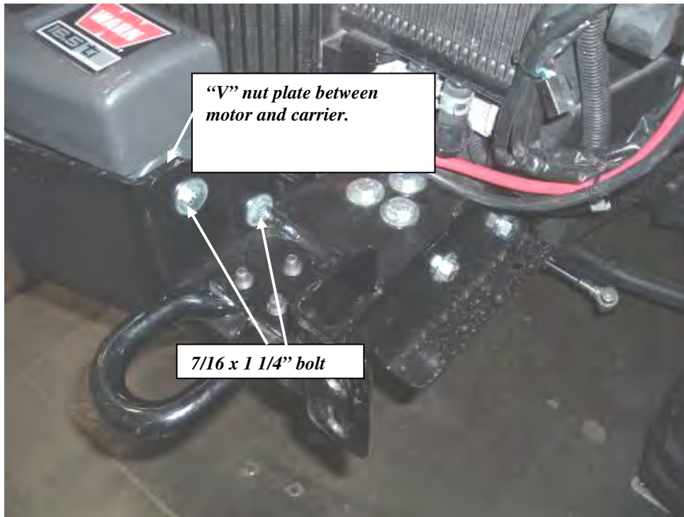
Figure 16: Winch Carrier installed.
