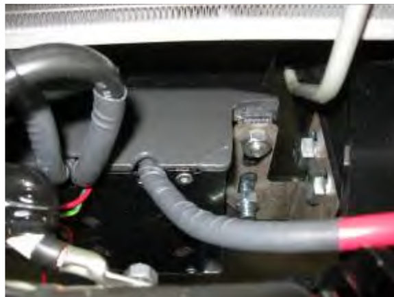
Figure 20: Control pack and Bracket Installation. (16.5Ti shown)
