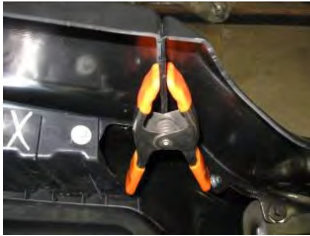
Figure 9: Clamp Top Cap to Center Skirt Piece.
