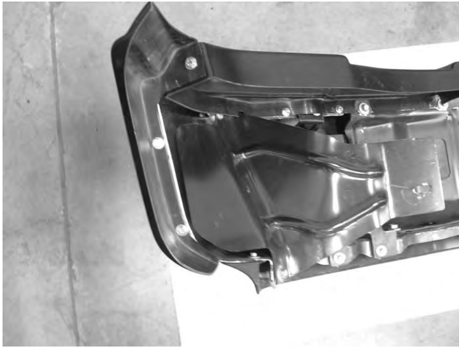
Figure 14 LH End Cap and Skirt installed
