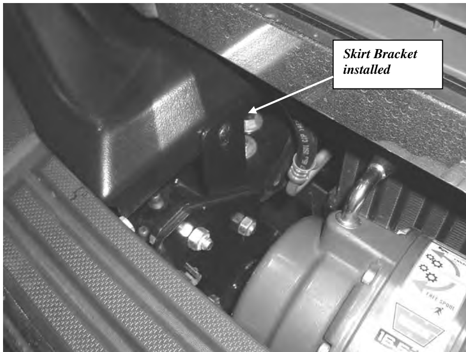
Figure 20 RH Skirt Bracket installed
