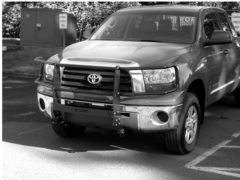
Figure 22 Installation complete-Vehicle shown with Brush Guards and Winch Carrier
