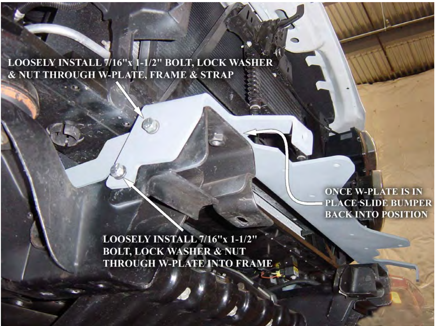
Figure 4: Install W-Plate.
