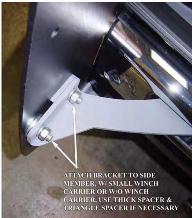
Figure 9a: Bracket Attachment w/o Winch Carrier
