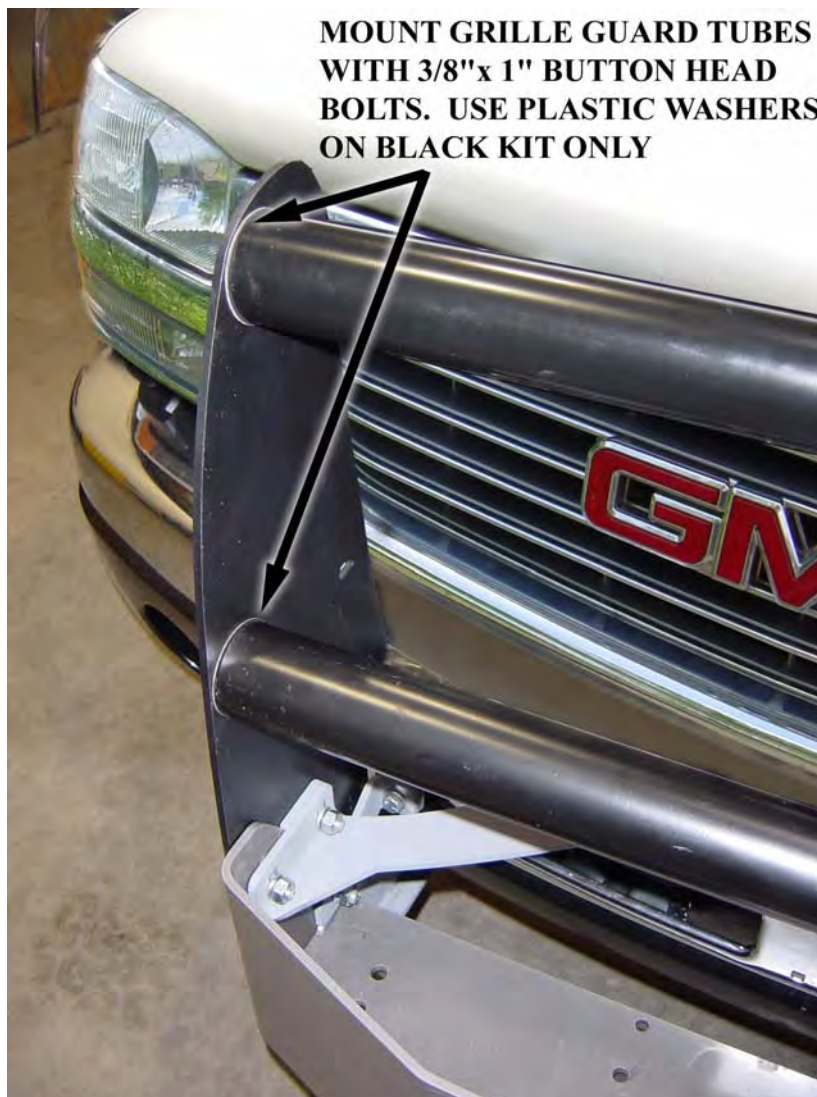
Figure 11: Mount Grille Guard Tubes.
