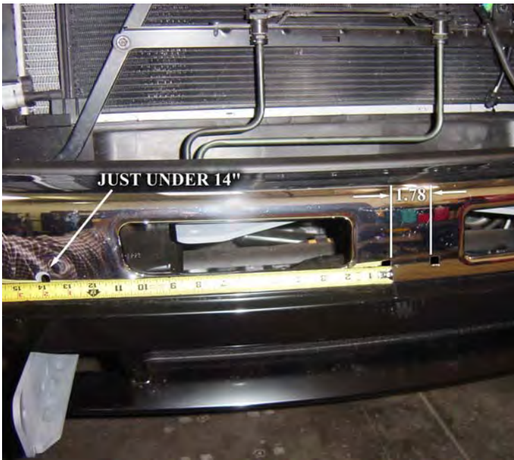
Figure 7a: Drilling holes for Bumper Bracket.
