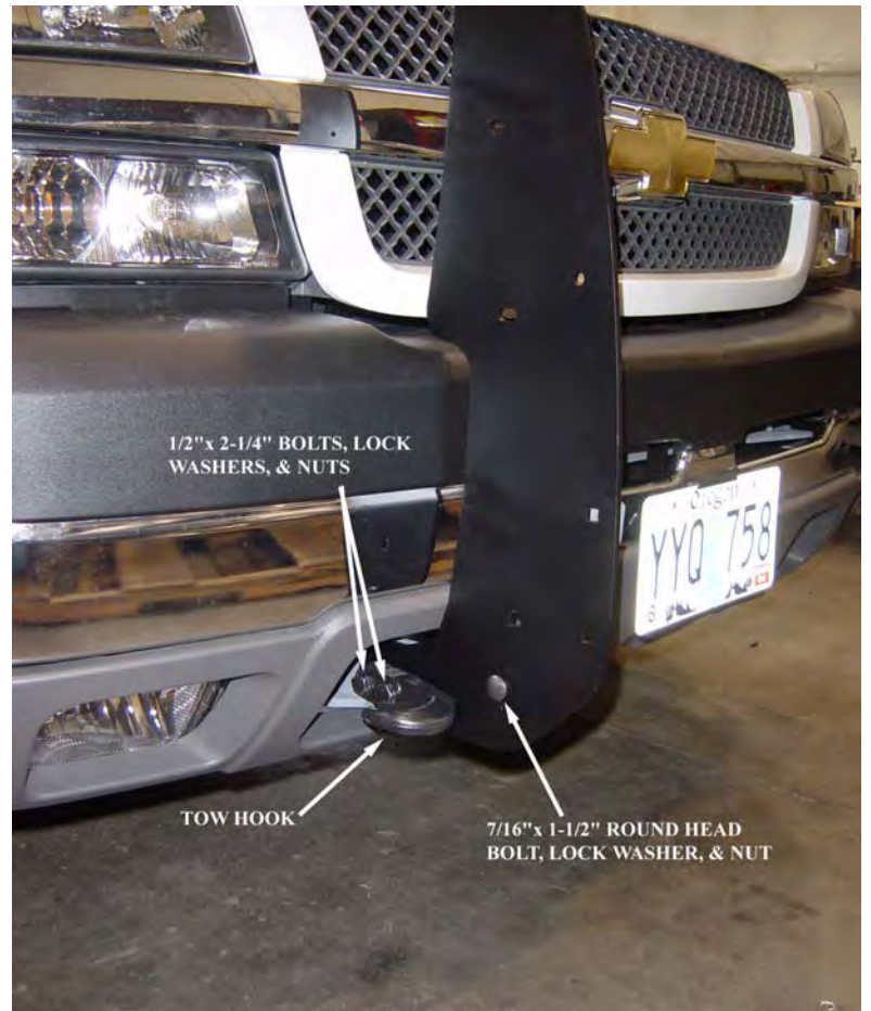
Figure 7: Side Member Installation.
