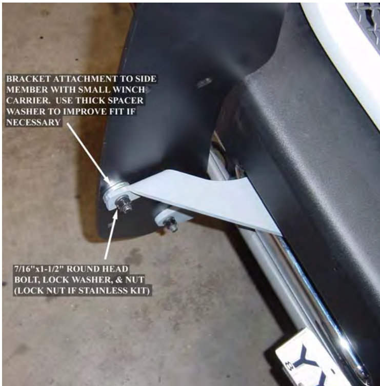
Figure 8a: Bracket attachment.
