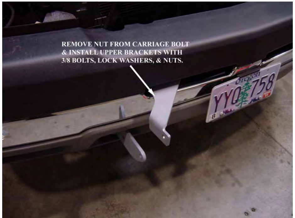
Figure 6: Install Upper Brackets.
