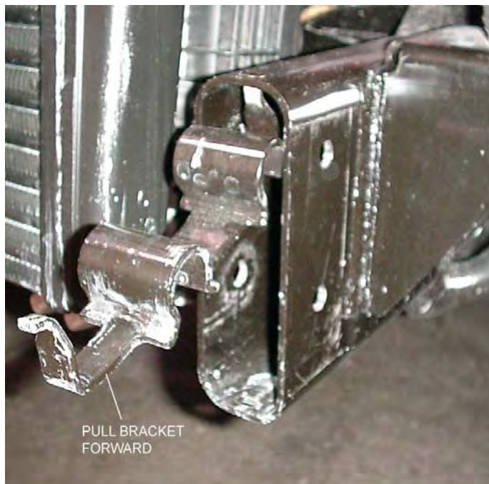
Figure 7 Left frame tube “anti-crush” brackets pried up for access inside the frame tube
