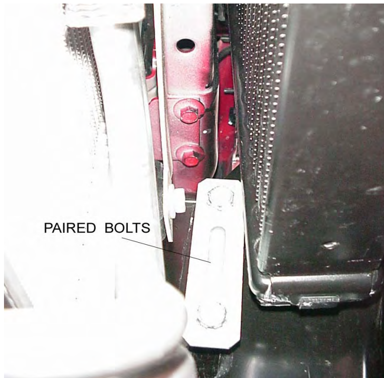
Figure 1 Bolts attaching bumper brackets to frame (viewed from center of vehicle, looking outward)
