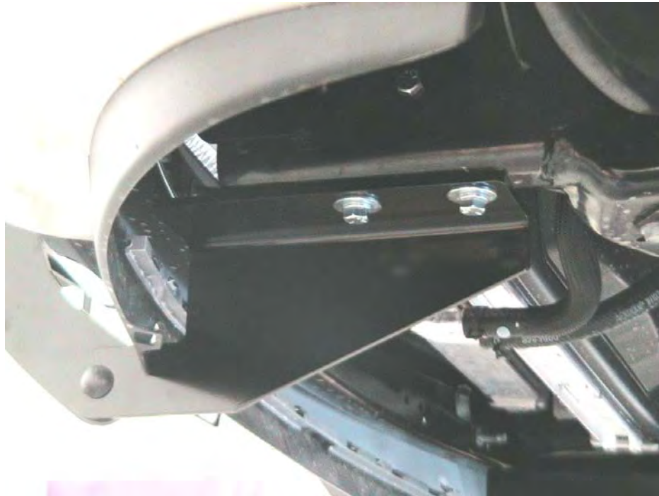
Figure 14 Vehicle frame and LH Lower Brace installed
