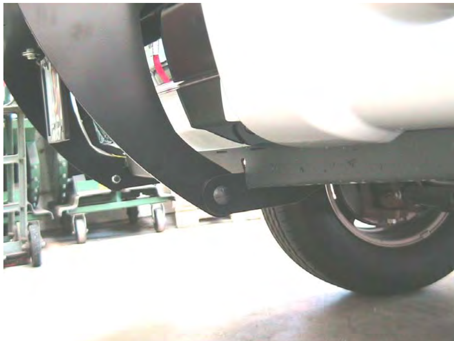
Figure 13 Side Members and Lower Braces installed
