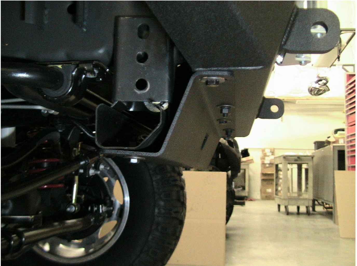
Figure 1: Skid Plate bolt locations
