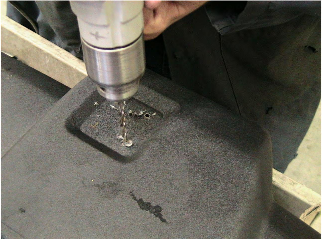
**Figure 3: Drill corners of tow hook cutout**
