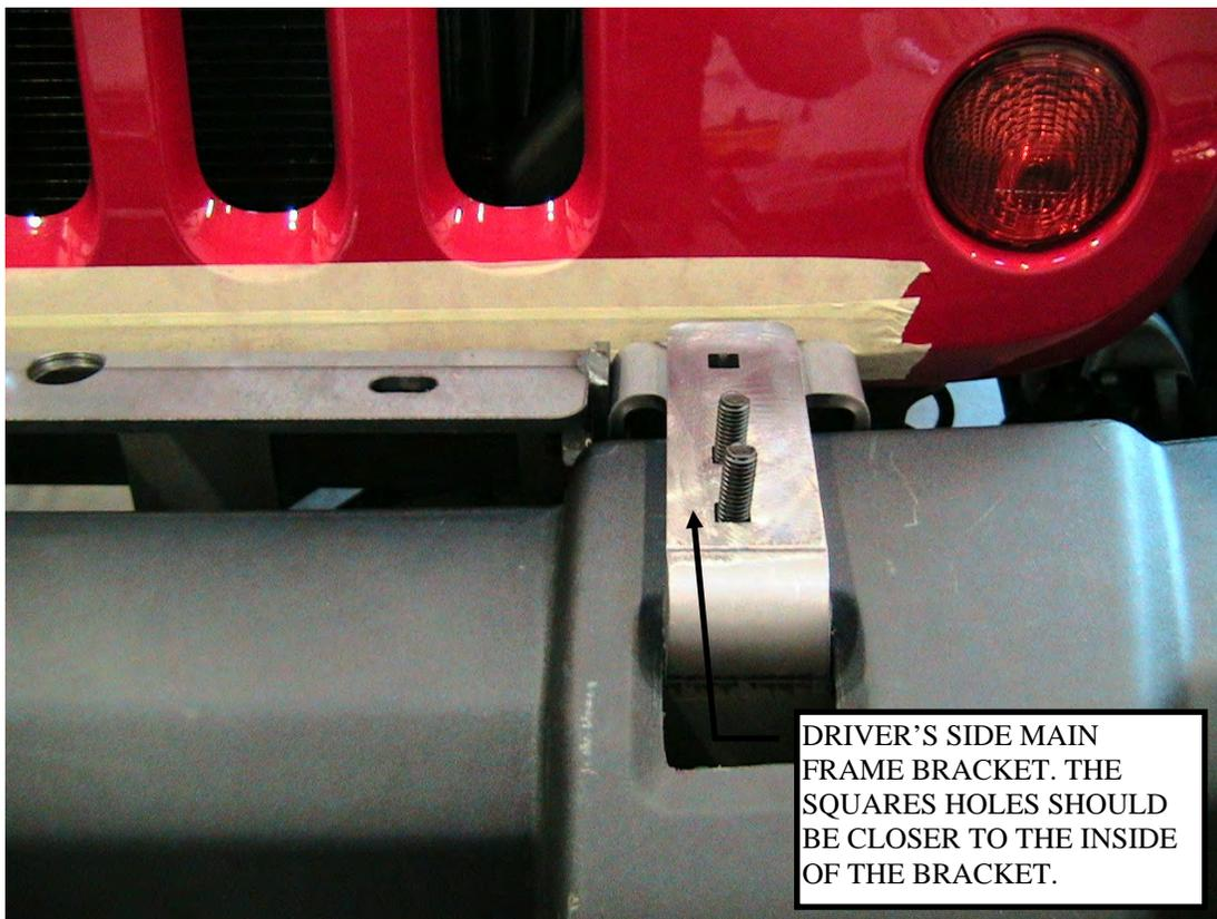
**Figure 9: Driver's side main frame bracket**
