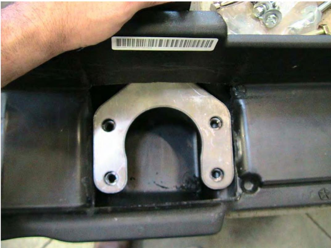
**Figure 5: Tow hook fitment into plastic bumper**
