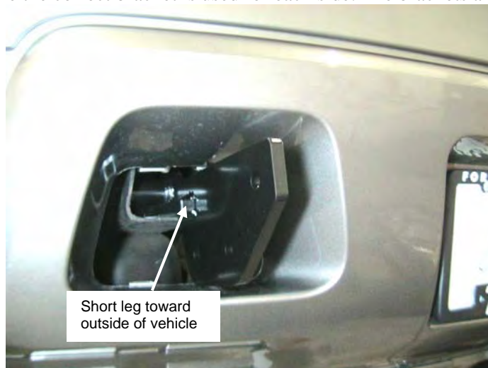
Figure 3 Frame Extension Installed
