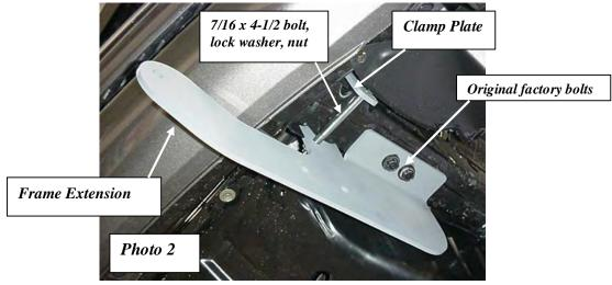
4. Install the Clamp Plates to the outsides of the frame using the 7/16 x 4-1/2" bolts, one over the top of the frame and one under the frame. Tighten securely. See **Photo 3**.
