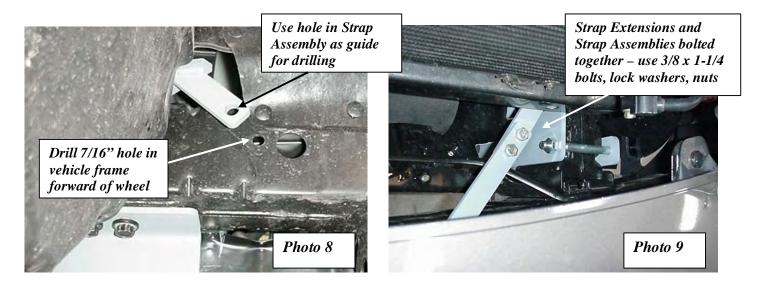
9. After the Strap sections are bolted together and to the Carrier, pull them back and position the tail section down tight against the frame. Mark the frame for drilling and drill a 7/16" hole.
