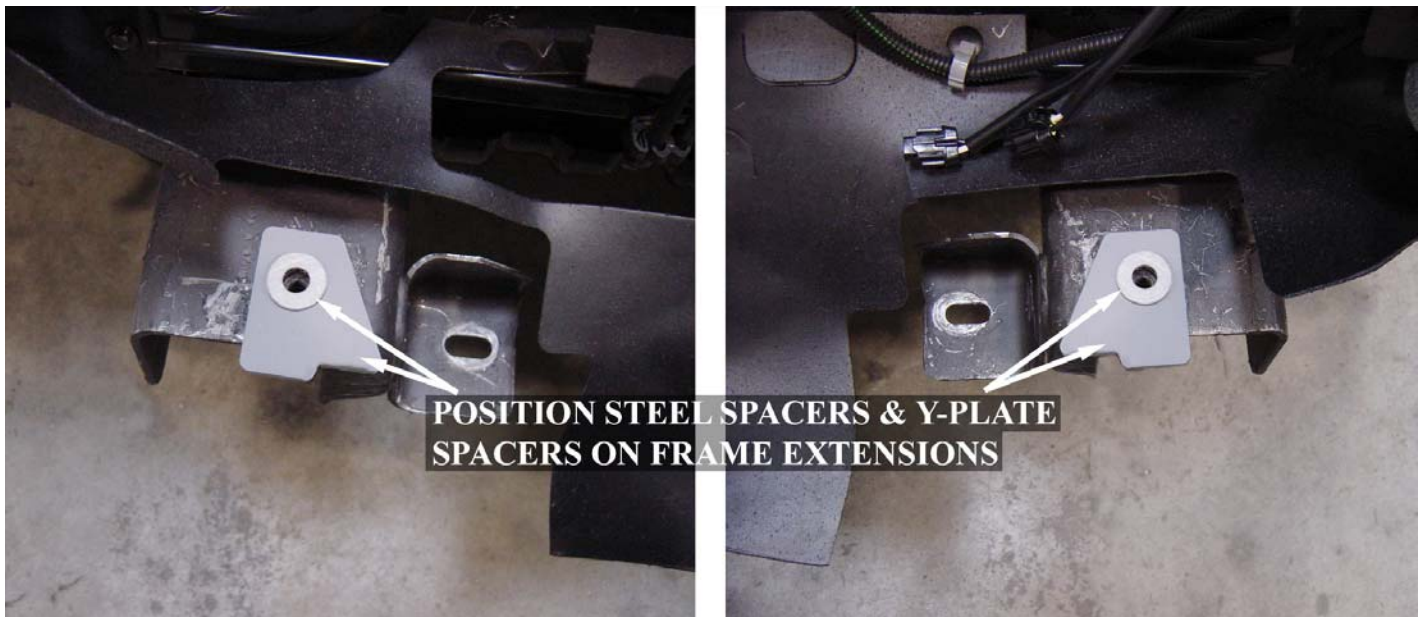
Figure 1: Place spacers on frame for drilling.
