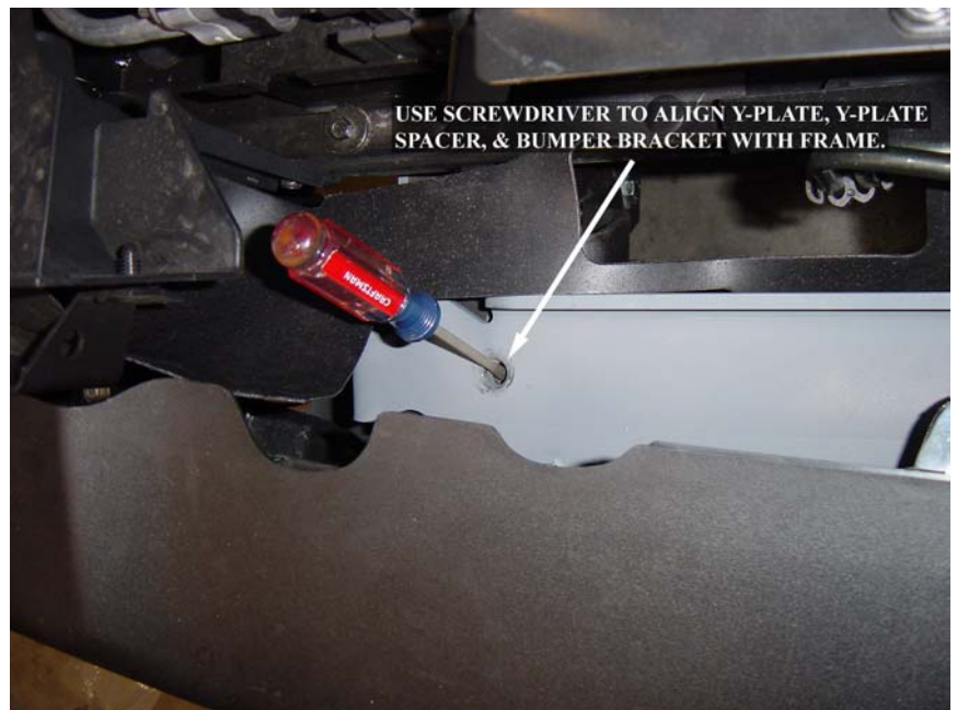
Figure 6b: Use screwdriver to align parts.
