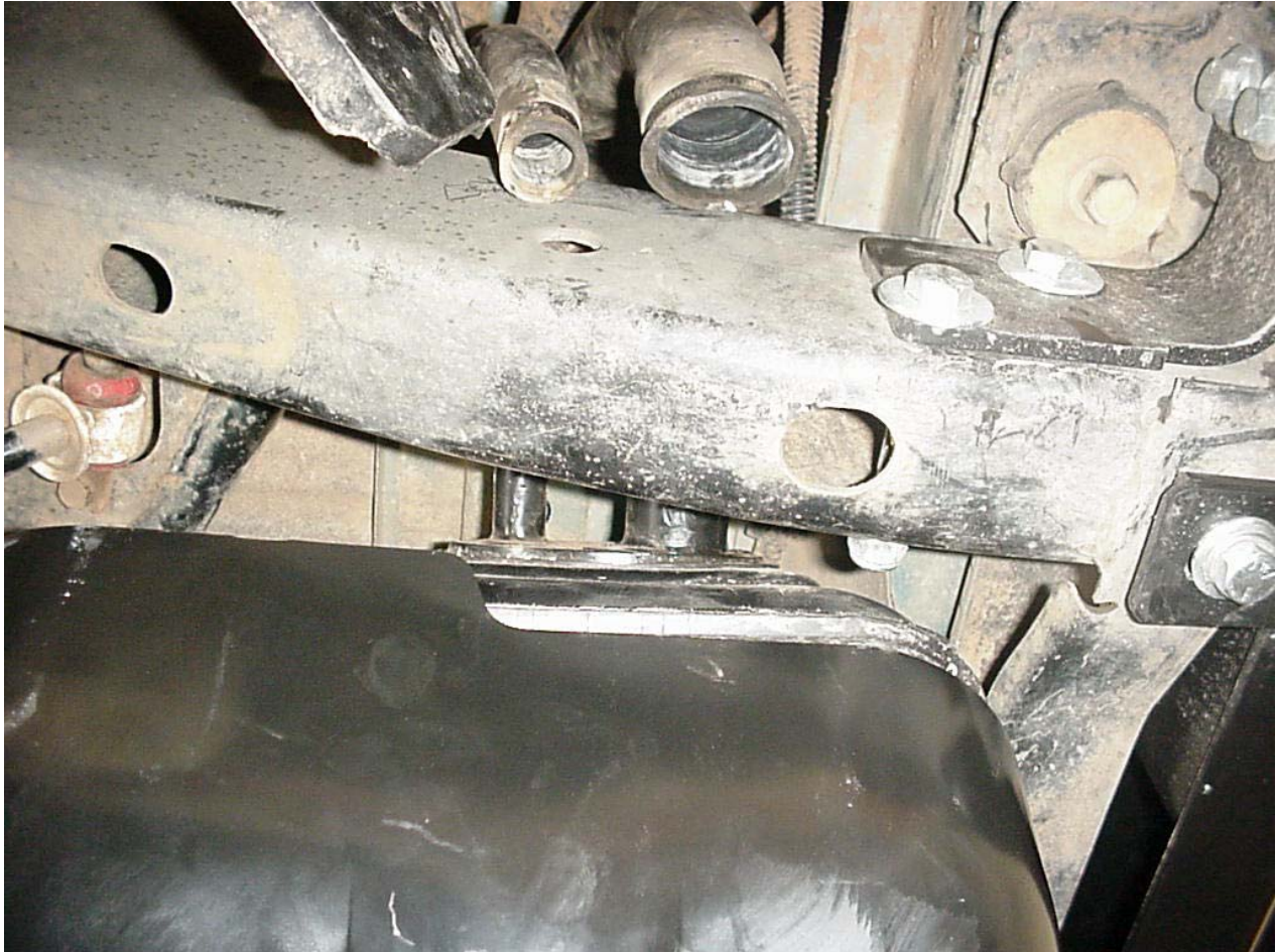
Figure 2: Fuel Filler and Overflow Hoses unhooked at tank.
