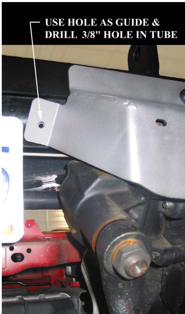
Figure 1: Drill location for 3/8" bolt.
