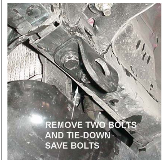
Figure 5. Left Side Tie-Down
