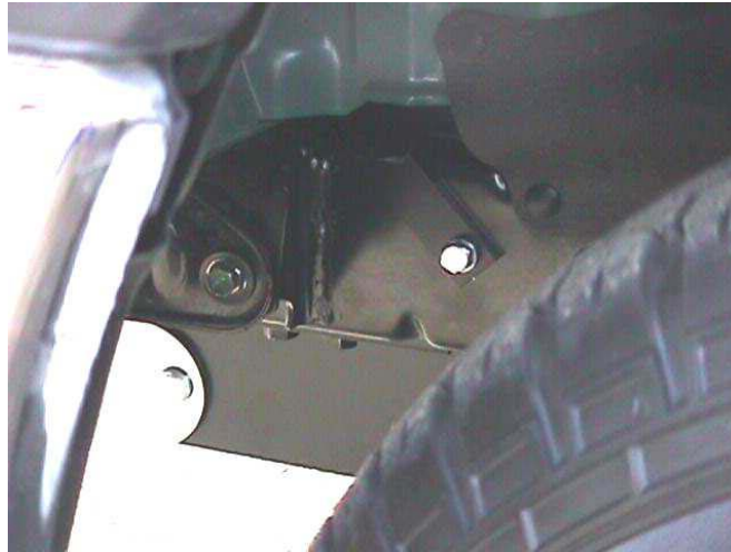
PHOTO 5 – strap assembly attached to frame
