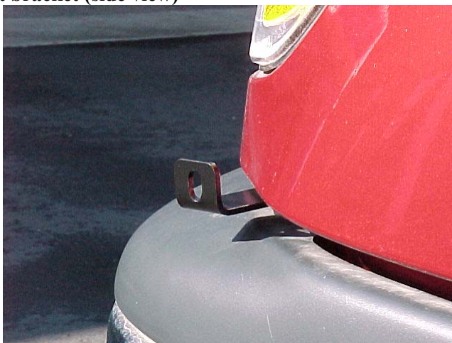
PHOTO 4 – brush guard support bracket (side view)
