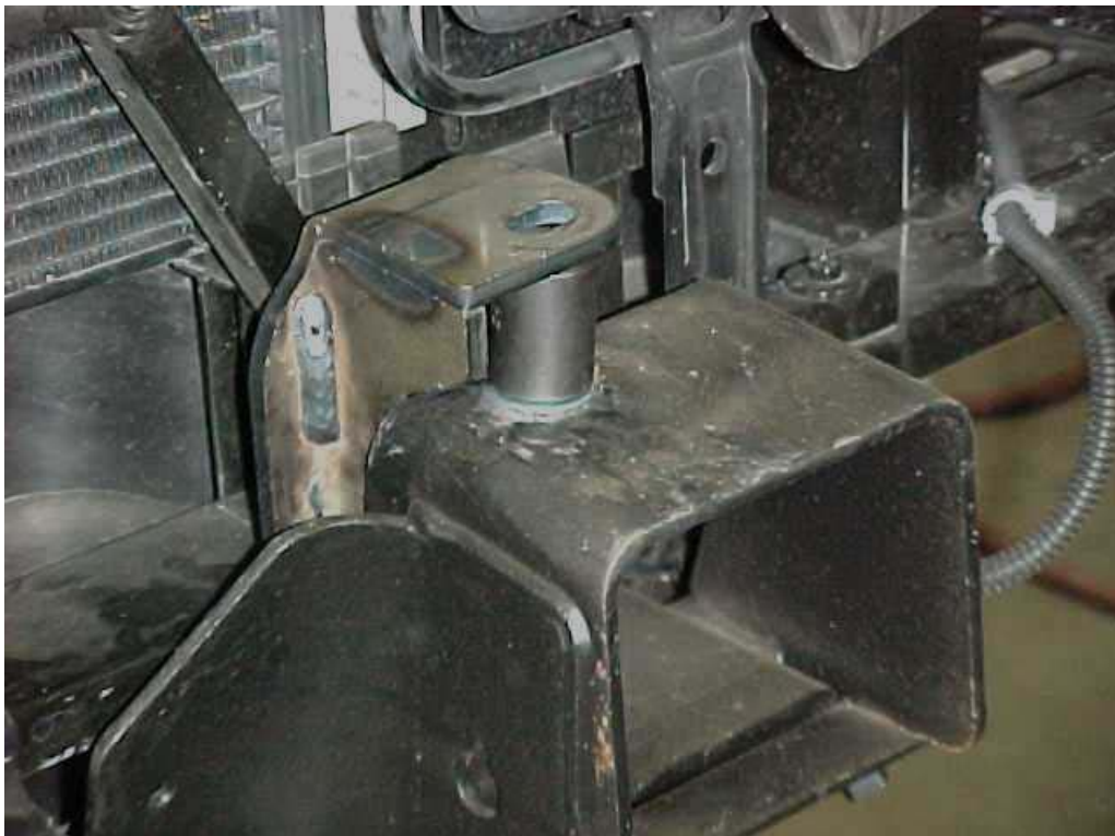
PHOTO 2 – brace assembly (NOTE: use shim washer (unplated) below the spacer to set the elevation. The shim represents the material thickness of the bumper.)
