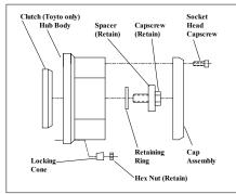
Some factory hubs are installed with locking cones, which can be difficult to remove.
