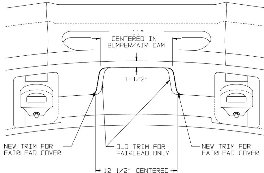
2. To install the Fairlead Cover, press it onto the vertical rollers of the fairlead then slide it up, inside the air dam. Be sure the cable hook does not prevent the cover from fully engaging the rollers.
