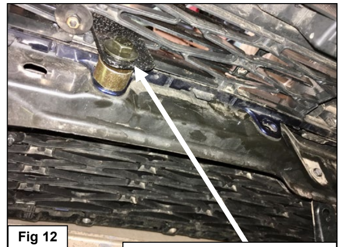
8mm x 30mm Hex Bolt (2) 8mm x 24mm Flat Washers 8mm Nylon Lock Nut
