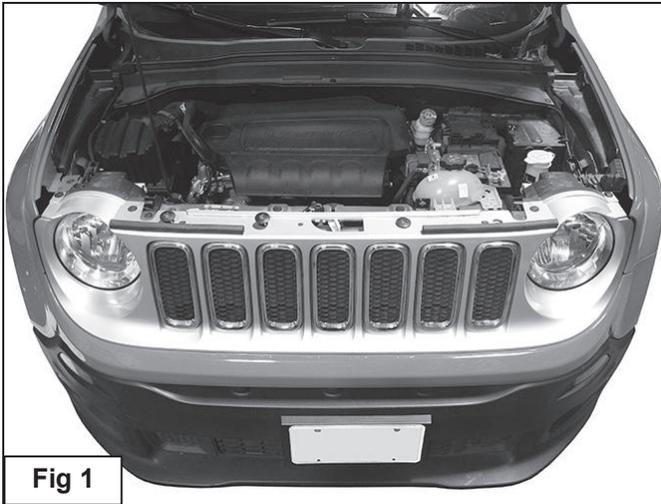
Remove hardware attaching the top of the grille to the radiator core support. Remove the hardware attaching the bottom of the bumper cover to the bottom of the radiator core support.
