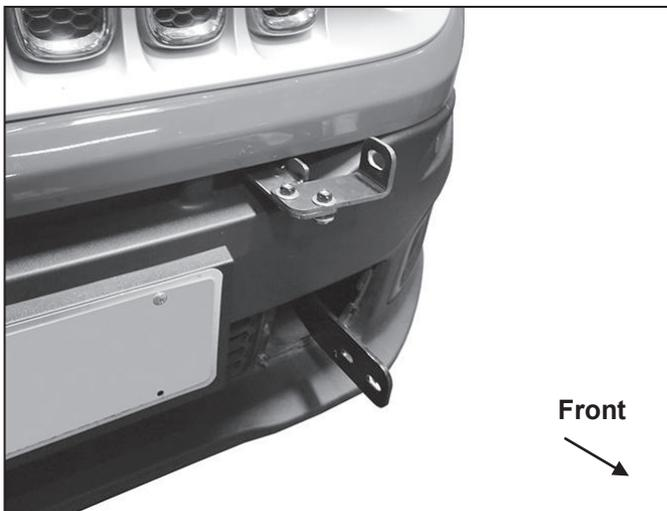
(Fig 18) Reinstall Top Support Brackets
