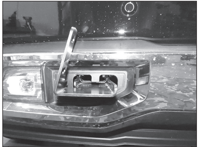
(Fig 11) Passenger/right side Bracket installed
