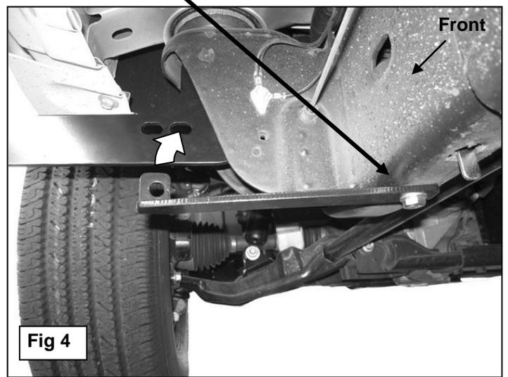
**IMPORTANT NOTE: 25-3500 Model Front Support Bracket Installation Pictured**
