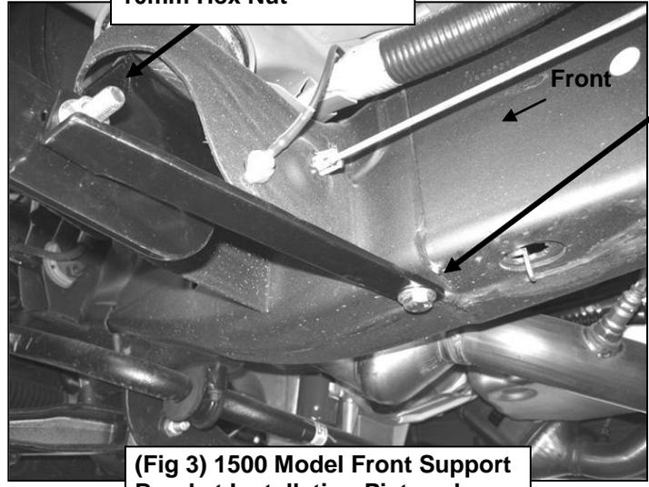
**(Fig 3) 1500 Model Front Support Bracket Installation Pictured**
