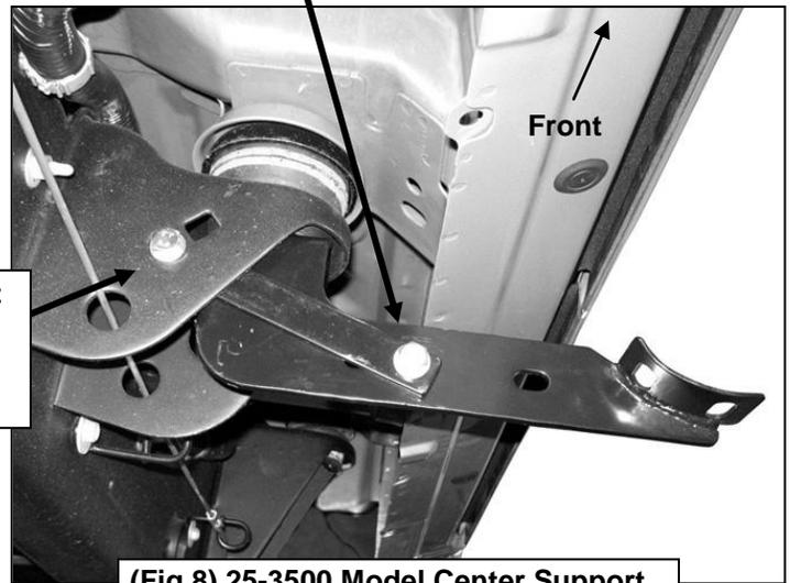
(Fig 8) 25-3500 Model Center Support Bracket Installation Pictured.
