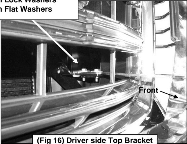
(Fig 16) Driver side Top Bracket installation pictured
