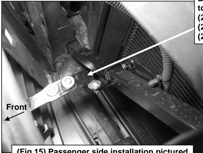
Bolt the Top Outer Bracket to the Inner Bracket with:
