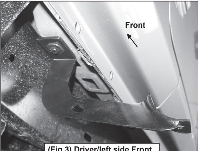
(Fig 3) Driver/left side Front Mounting Bracket installed
