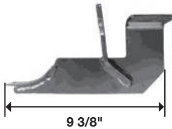
Figure 3B - Passenger-side front mounting bracket
